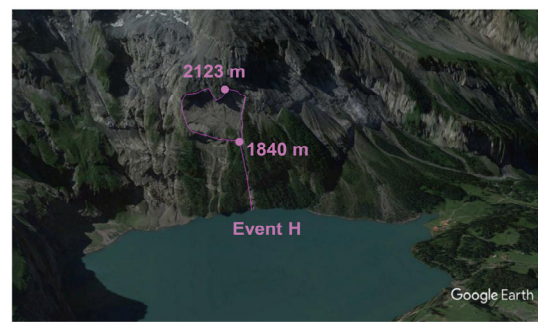
Figure S4. Detailed aerial images with scarp niches, elevations and assumed travel paths.
