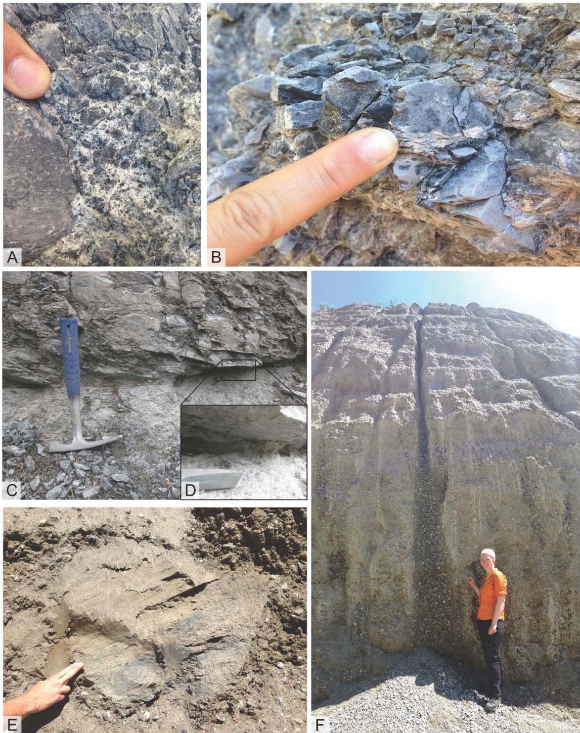
Figure 5: Examples of energy-related features in deposits of the Flims Rock Avalanche (Switzerland): (A) Shattering into cube-like, sharp-angled fragments of different size (cm-dm) in dark grey Helvetic limestone, secondarily cemented with white matrix of rock powder. (B) 'Snapshot' of pulverization with multiple grain-internal layers of micro-shearing. (C) and (D) Grinding within a shear zone. (E) Entrained lump of lake sediment in the Bonaduz gravel deposits. (F) Vertical Pavoni pipes indicate rapid water discharge after deposition (person for scale).
