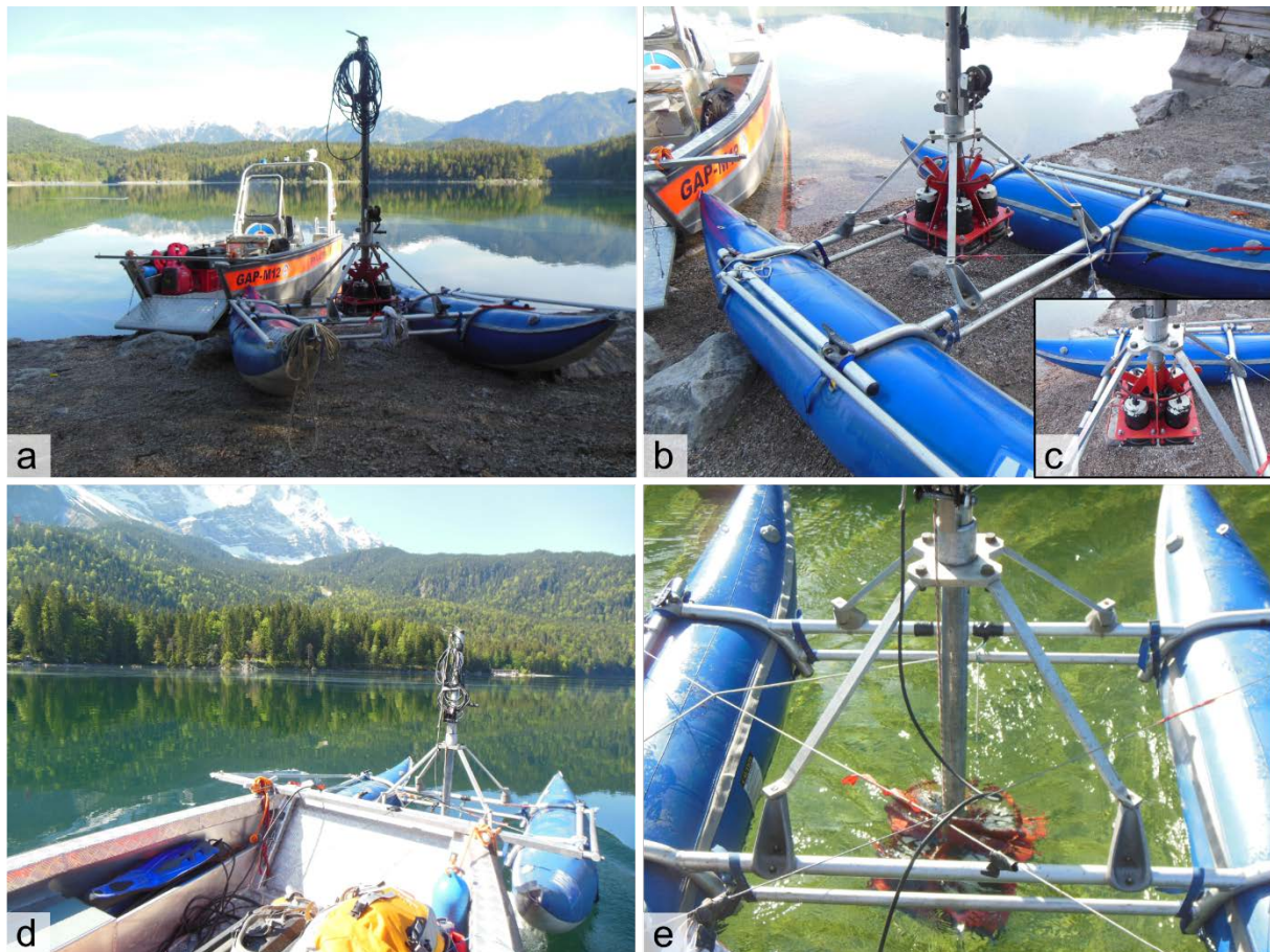
Figure 7: Setup for a reflection seismic survey showing a) the boat and the catamaran, b) equipped with a seismic source (red), which c) contains four piezo crystals (black / white). During operation, d) the catamaran is navigated in front of the boat, with e) the pinger positioned directly below the water surface.
