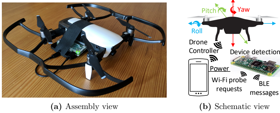
Figure 4.4: Drone platform for autonomous device management [7]
