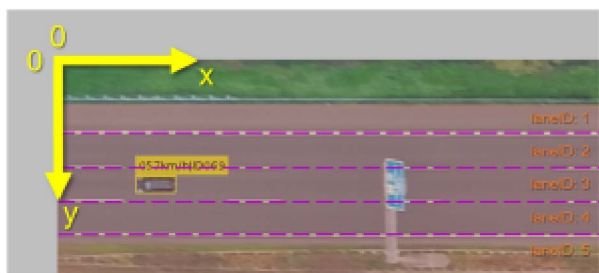
Fig. 4. The coordinate system of highD dataset
