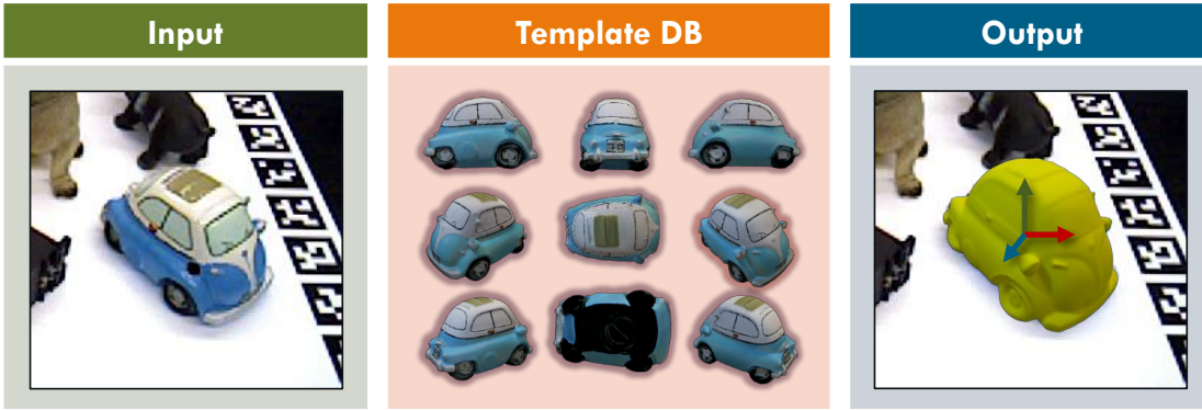
Figure 2.10: Template-based methods. A database of templates covers possible object views. Each template is compared to the input image and the best fitting template is used as a pose estimate.
