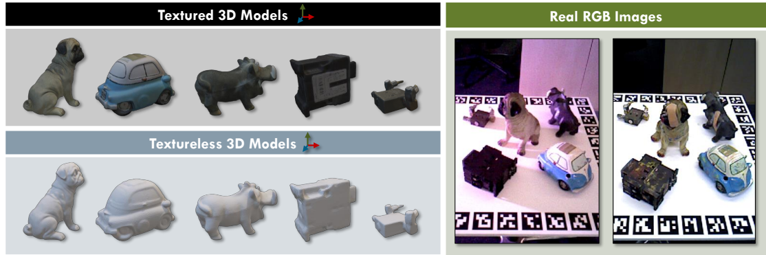
Figure 1.3: Domain gap. Synthetic data are very different from real images coming from commodity sensors not only due to the sensor-specific properties, but also due to external illumination and object appearance changes. The problem becomes even more difficult when objects have no texture.
