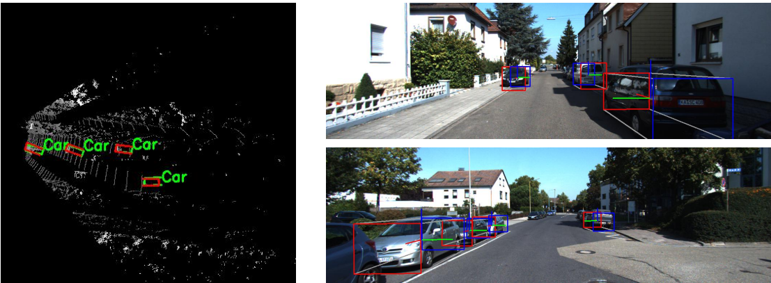
Figure 5.10: Detections from the autolabel-trained detectors. We draw local 3D frames to identify correct orientation.
