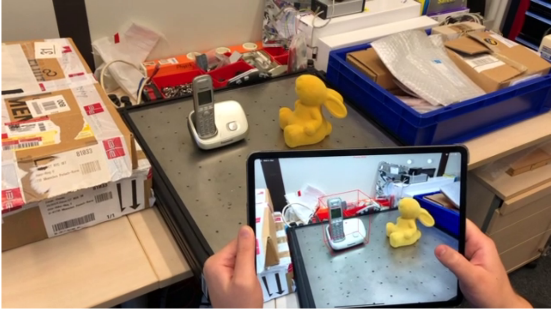
Figure 1.1: 6D pose estimation on a tablet. Our RGB dense pose object detector (DPOD) from Chapter 4 estimates 6D pose of the object in real time running on a tablet.
