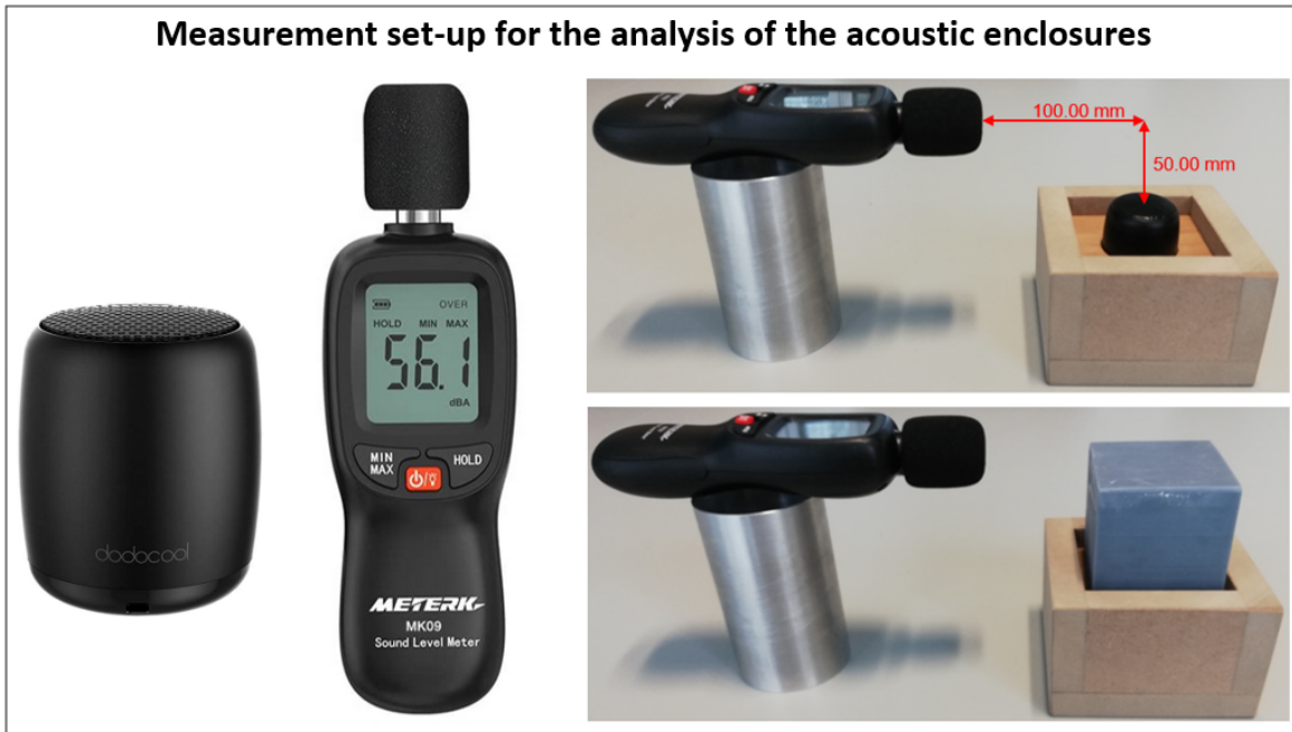
Figure 5.2: Bluetooth speaker from dodocool ® , sound level meter MK09 ® from Meterk ® and loudspeaker box (Dodocool, n.d.) (Meterk, n.d.)
