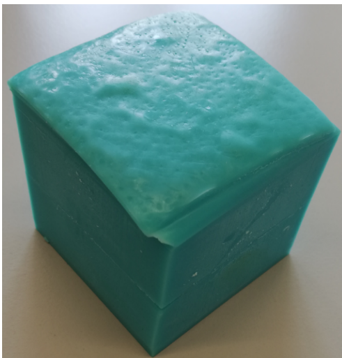
Figure 3.12: Manufacturing defects due to incorrect pressure settings
