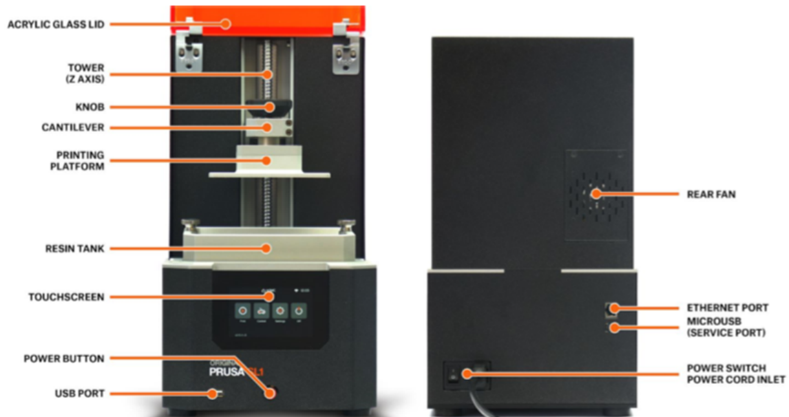
Figure 3.10: 3D printer Prusa SL1 ® (PrusaResearch, 2019)
