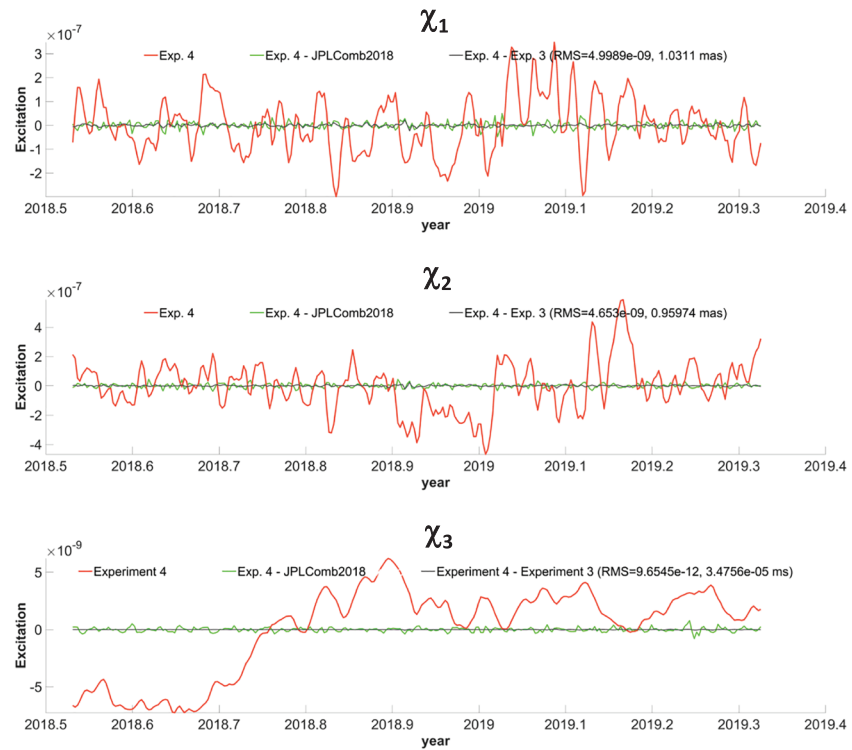
Figure 6. Geodetic angular momentum functions GAM from a combination of GNSS and SLR at observation level (experiment E4; red) and residuals after subtracting experiment E3 (gray) and JPL-Comb2018 (green), for \chi_1 (top), \chi_2 (middle), and \chi_3 (bottom). Excitation functions GAM and EAM are unitless. For better comparison with Figure 2, RMS values are also given milliarcseconds [mas] for the equatorial components \chi_1 and \chi_2 , and milliseconds [ms] for the axial component \chi_3 .
