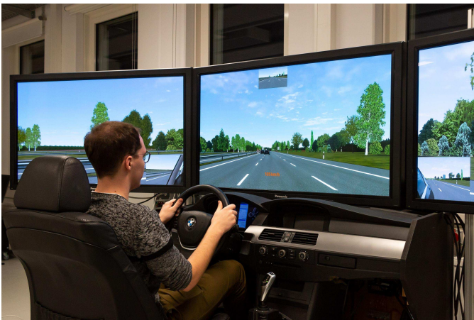
Fig. 10: The BMW driving simulator consisting of a cockpit and three monitors visualizing the environment.
