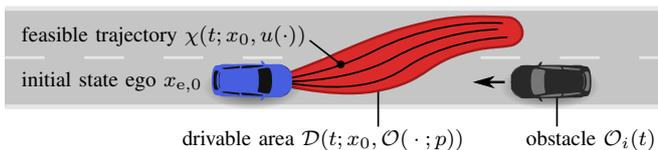
Fig. 6. Example of a drivable area for the time interval  $[t_0, t_f]$ .
