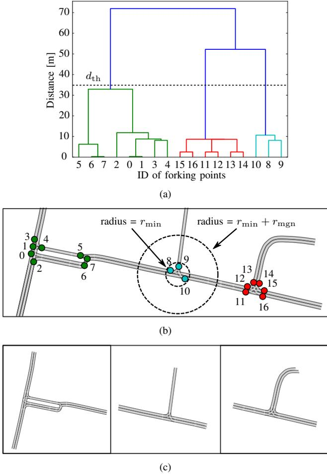
Fig. 4. (a) Dendrogram of the clustering result. Three clusters are generated with  $d_{th}$  set to 35 meters. (b) Forking points within one cluster have the same color.  $r_{mgn}$  is set to 15 meters. (c) Intersections extracted from the input lanelet network.
