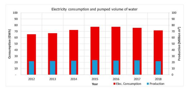
**Figure 9.** Total production (in the system) and Energy consumption of Wadi Al Arab wells and the three pumping stations 2012–2017.
