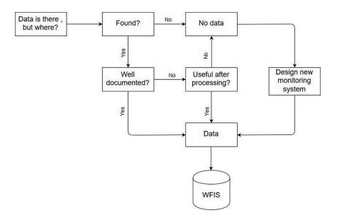
Figure 6. Schematic diagram for the followed processes to build the wellfield information system (WFIS).
