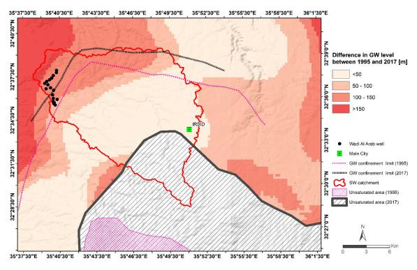
Figure 5. The decrease in the saturated thickness between the year 1995 and 2017.
