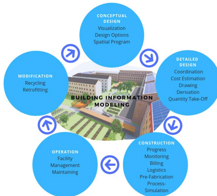
Figure 1.1: Information exchange during the whole life time of a built asset. (Speiser (2019), based on Borrman et al. (2018))
