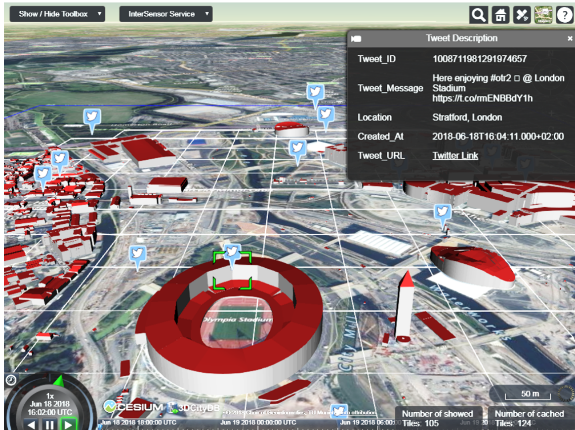
Figure 8.10: Joint visualisation of geo-tagged tweets retrieved by the InterSensor Service along with CityGML based 3D building objects in the district Queen Elizabeth Olympic Park, London. Screenshot taken from the 3DCityDB-Web-Map application.
