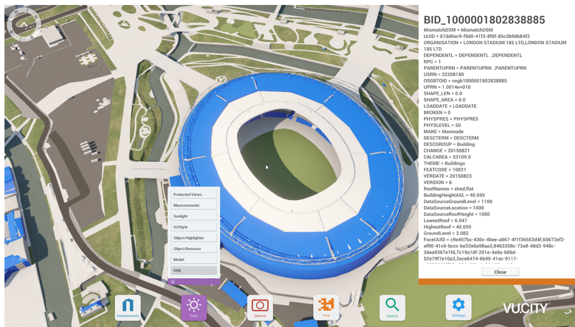
Figure 8.13: Illustration of the SDDI functionalities with an external visualisation platform. The thematic attributes of the CityGML model are parsed and retrieved by the VU.City platform. Screenshot taken from the VU.City application.
