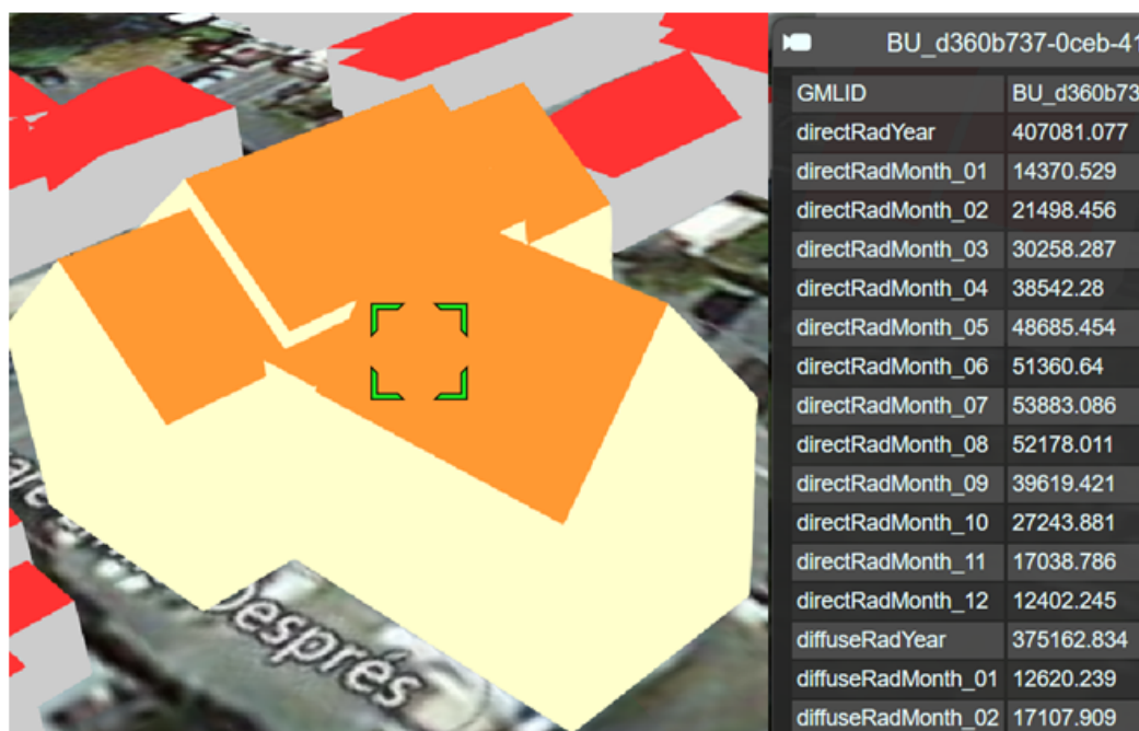
Figure 2.5: Tabular representation of monthly irradiation values of a building in Rennes, France. Screenshot taken from the 3DCityDB-Web-Map-Client.
