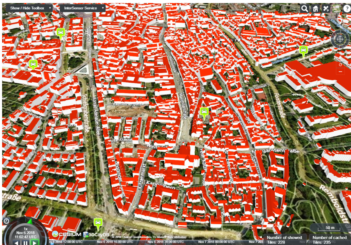
Figure 8.11: Joint visualisation of available rental car information being retrieved by the InterSensor Service along with CityGML based 3D building objects in the city of Augsburg in Germany. Screenshot taken from the 3DCityDB-Web-Map application.
