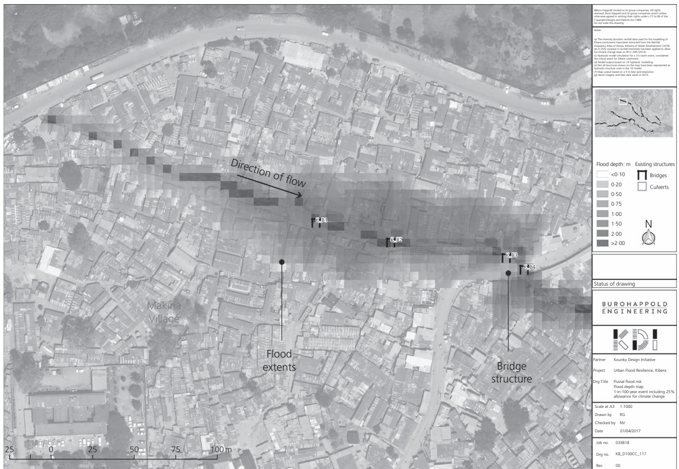
Figure 9. Model outputs for a 1-in-100-year flood extents demonstrating localised flooding driven by a bridge structure in the Makina village of Kibera (source: BuroHappold Engineering)
