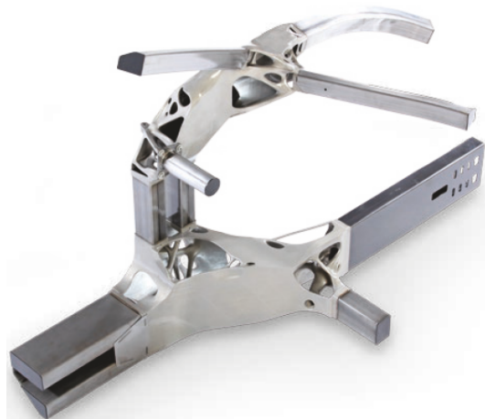
(b) Hybrid space frame concept by LZN, EDAG, BLM and Concept Laser (LZN (2017)).
