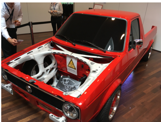
(a) 3D-printed VW Caddy front-end structure developed within the 3i-PRINT project.
