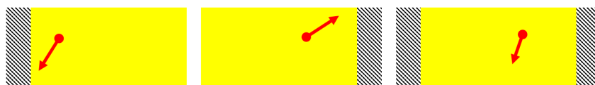
Figure 6.15 Three types of boundary conditions used in the sampling process (Bujny et al. (2018)). The nodes in the FE mesh can be fixed on the left, right or on both sides. In all of the three cases, a single point load is applied in a random direction and at a random position within the design space.
