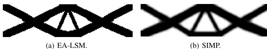
Figure 7.4 Comparison of the best topology obtained with EA-LSM and SIMP (Andreassen et al. (2011)) for the transverse bending problem.
