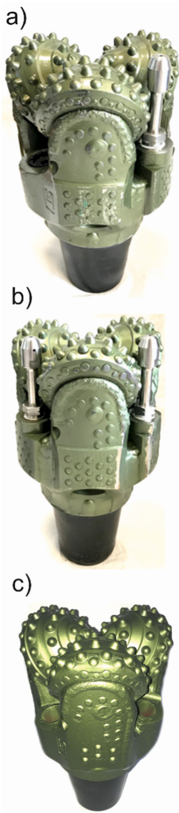
Fig. 4. Novel drill bits: a) one-nozzle bit and b) two-nozzle bit and c) the baseline bit.
