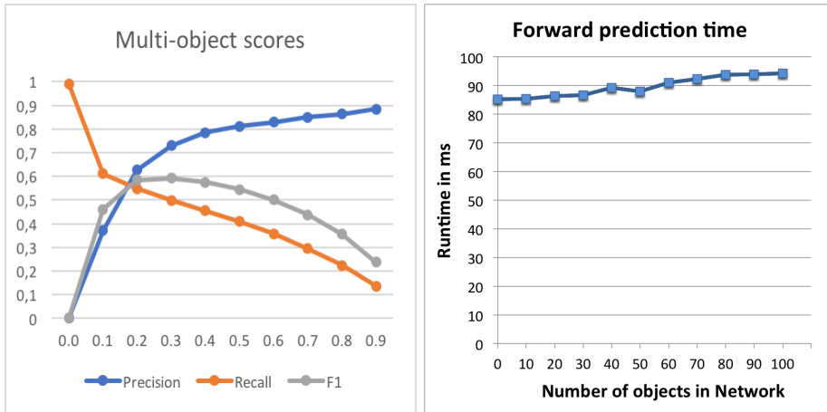
Figure 7.8: Left: Detection scores on the multi-object dataset for a different global threshold. Right: Runtime increase for the network prediction with an increased number of objects.
