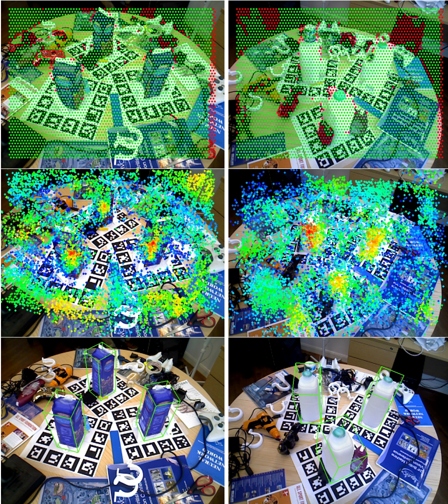
Figure 6.9: Scene sampling, vote maps and detection output for two objects on the Tejani dataset. Red sample points were skipped due to missing depth.
