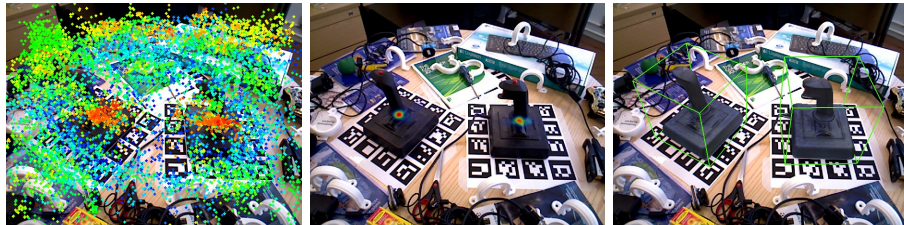
Figure 6.5: Starting with thousands of votes (left) we filter and retrieve intermediate local maxima (middle) that are further verified and accepted (right).
