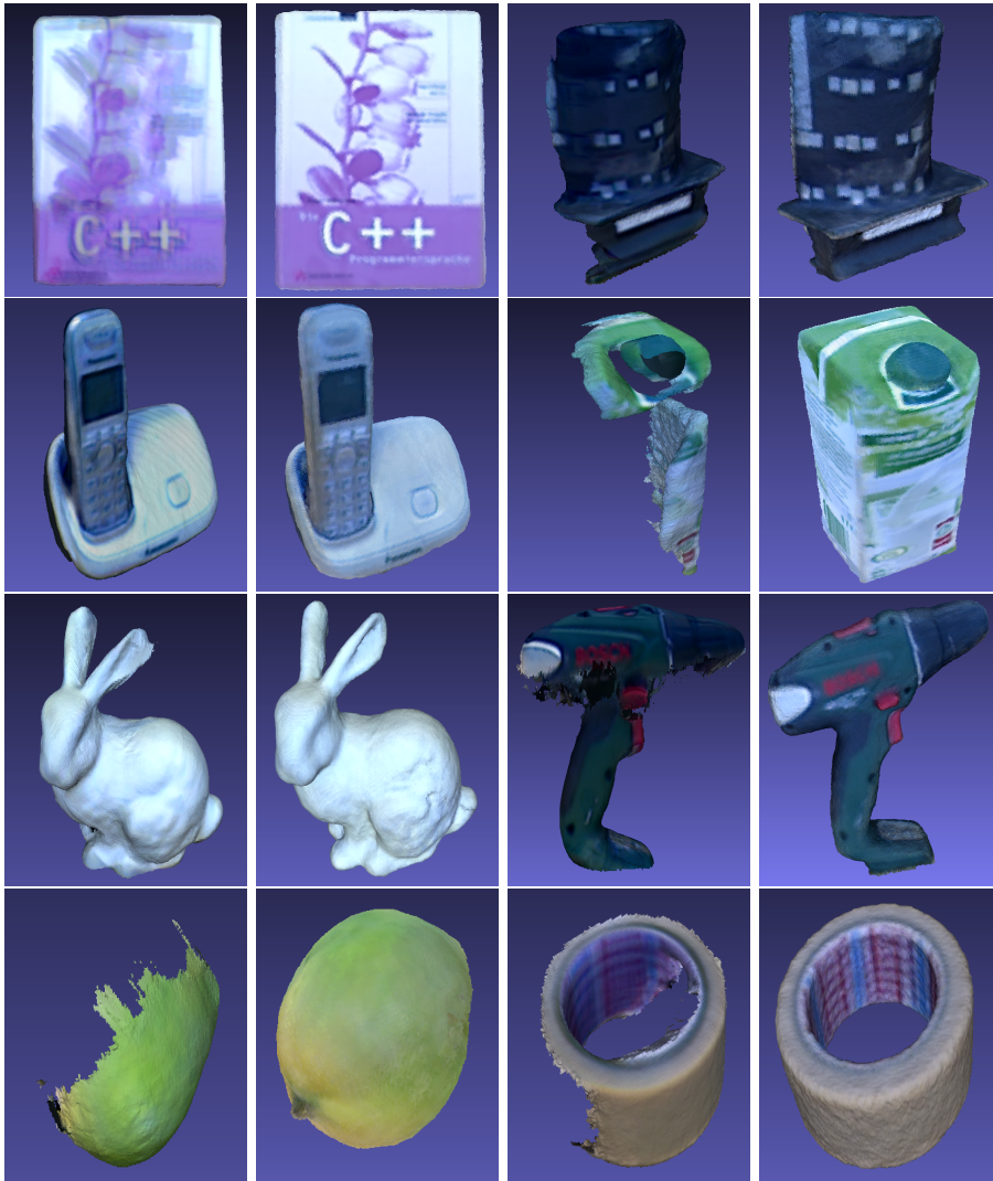
Figure 3.3: Reconstructions of the eight objects. Each pair depicts the results from KinectFusion on the left and our approach on the right. We clearly recover richer texture as well as geometry. We are even able to fully reconstruct symmetric objects like the tape object or geometrically poor objects like the mango. Also note the textural fidelity of mostly every object that was reconstructed with our method.
