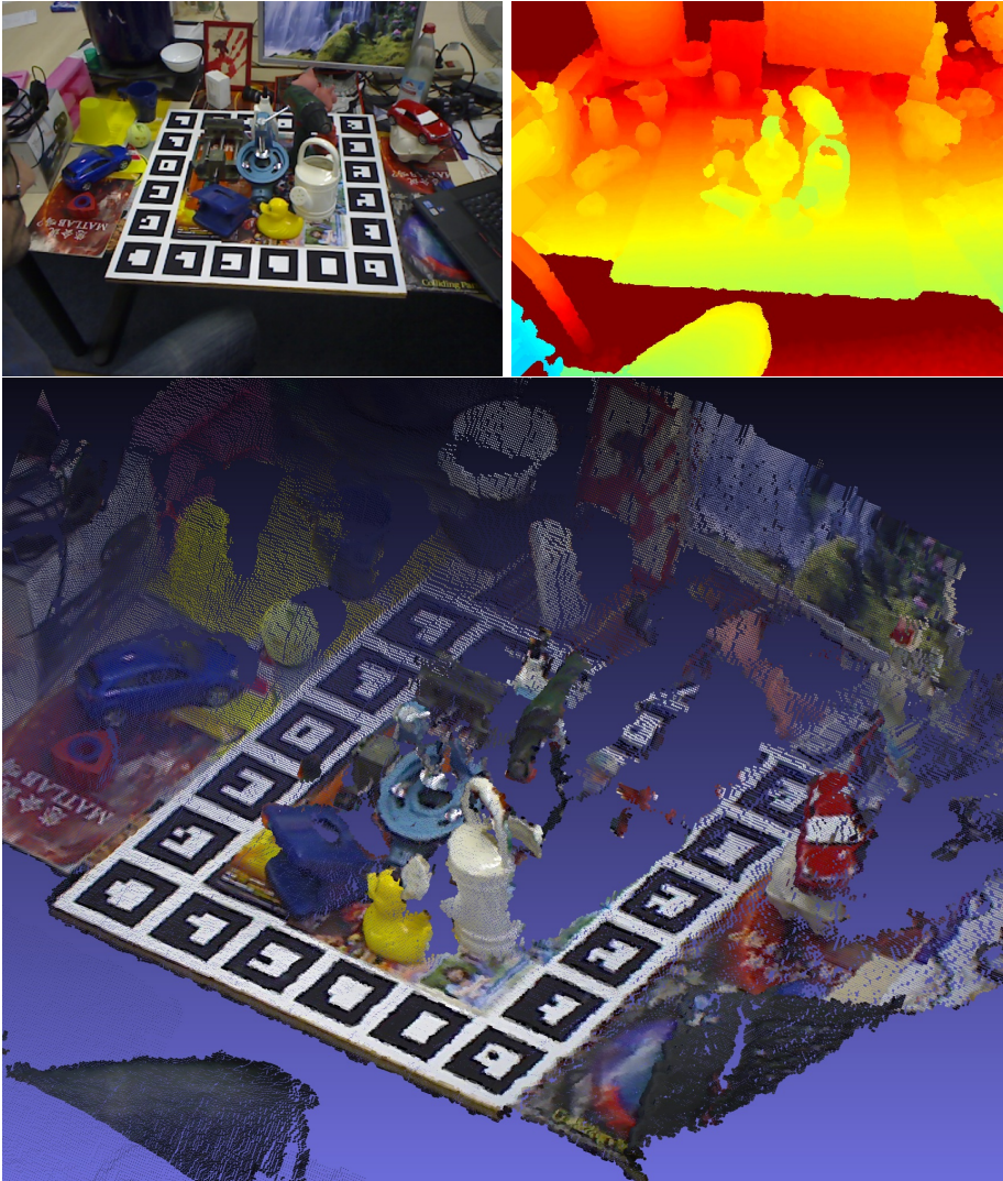
Figure 2.2: A frame from the LineMOD dataset [Hinterstoisser et al., 2012a]. The top row shows a registered image pair of color and depth. The depth channel is presented as a heatmap for better visualization. The image at the bottom shows the colored point cloud data produced from the application of Eq. 2.6 and slight rotation for easier interpretation. Such data allows for better reasoning about relations in metric scale, occlusions and more generally, whether space is occupied or not. Additionally, it enables reliable estimation of scene normals and surface curvature.
