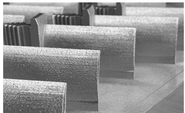
(b) Varying levels of defect for different blades
