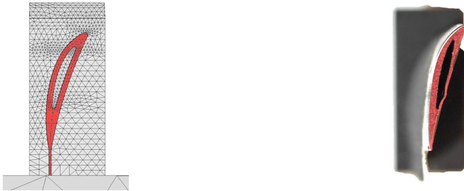
(a) Nominal geometry (meshed) on the build plate
