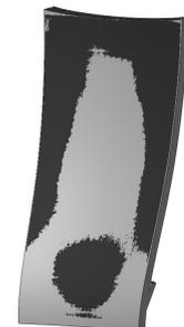
(b) Initial (light) and deformed (dark) panel geometry after LBM (see also Figure 5.7 on page 59)
