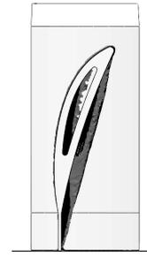
(b) Initial (light) and deformed (dark) blade geometry after LBM
