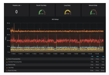
Fig. 2: Time evolution of the QoS KPIs: packet loss and delays of the sensor, controller, network, round-trip, and control loop.
