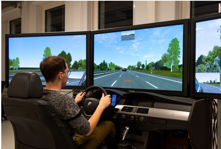
Figure 6.20: BMW driving simulator. A study participant steers the simulated vehicle in a safety-critical scenario of the user study [5]. The longitudinal motion is automated by an adaptive cruise control system (ACC), which is supervised by the proposed fail-safe motion planning technique. We compare the passengers' comfort and feeling of safety by enabling and disabling the verification layer for different runs of a scenario.
