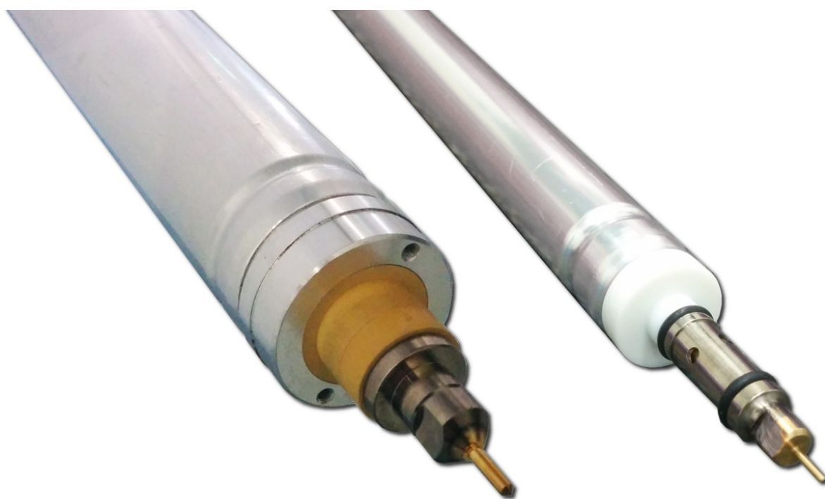
Figure 2.4: MDT (left) and a sMDT (right) with their endplugs signal caps [22].
