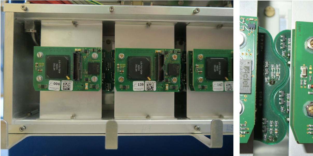
(a) An opened BMG Faraday cage. The gas distribution system is hidden behind the shielding plates between the high voltage signal readout board and the active ASD board.
