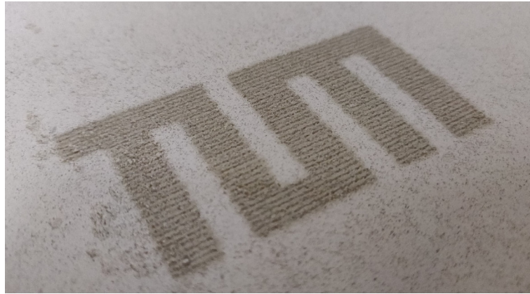
Figure 5: Close up of a printed layer with visible individual printed lines. Printed image dimensions: 68 mm x 35 mm
