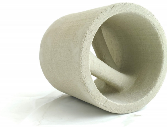
Figure 8: 3D-printed pipe segment with internal trusses
