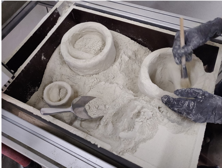
Figure 7: Printed parts during excavation
