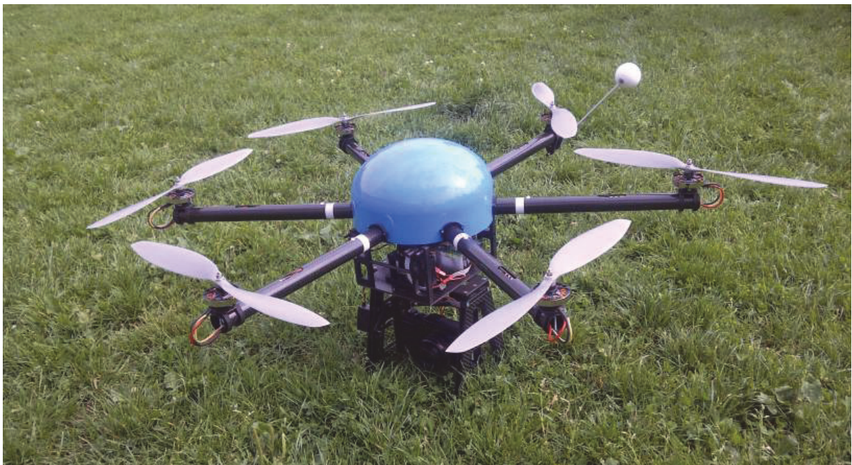
Figure 7 MAC2 from cooperation Stix-Neuner-Donauer from Austria, a MAV with six propellers (Ott).
