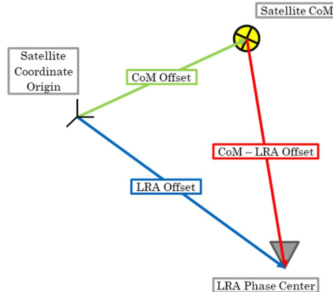
Positions of the LRA and DORIS phase centers in the inertial reference frame depend on the satellite orientation in space
