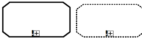
Figure 2.3.: Planned and discretionary Stage notated in CMMN (Object Management Group, 2016).
