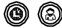
Figure 2.6.: Timed event listener and User event listener notated in CMMN (Object Management Group, 2016).
