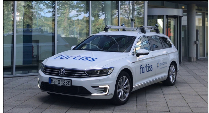
Fig. 2: The fortuna autonomous driving vehicle demonstrator: a modified VW Passat with Lidar sensors and antennas on the roof rack, additional cameras inside the vehicle and additional radar sensors integrated in the bumpers.
