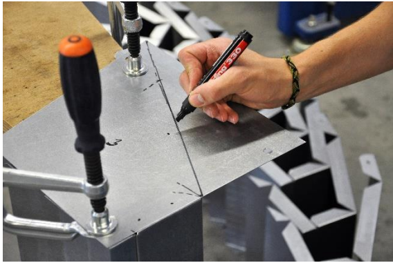
Figure 5-29: Estimating the flap measurements and positioning the bores
