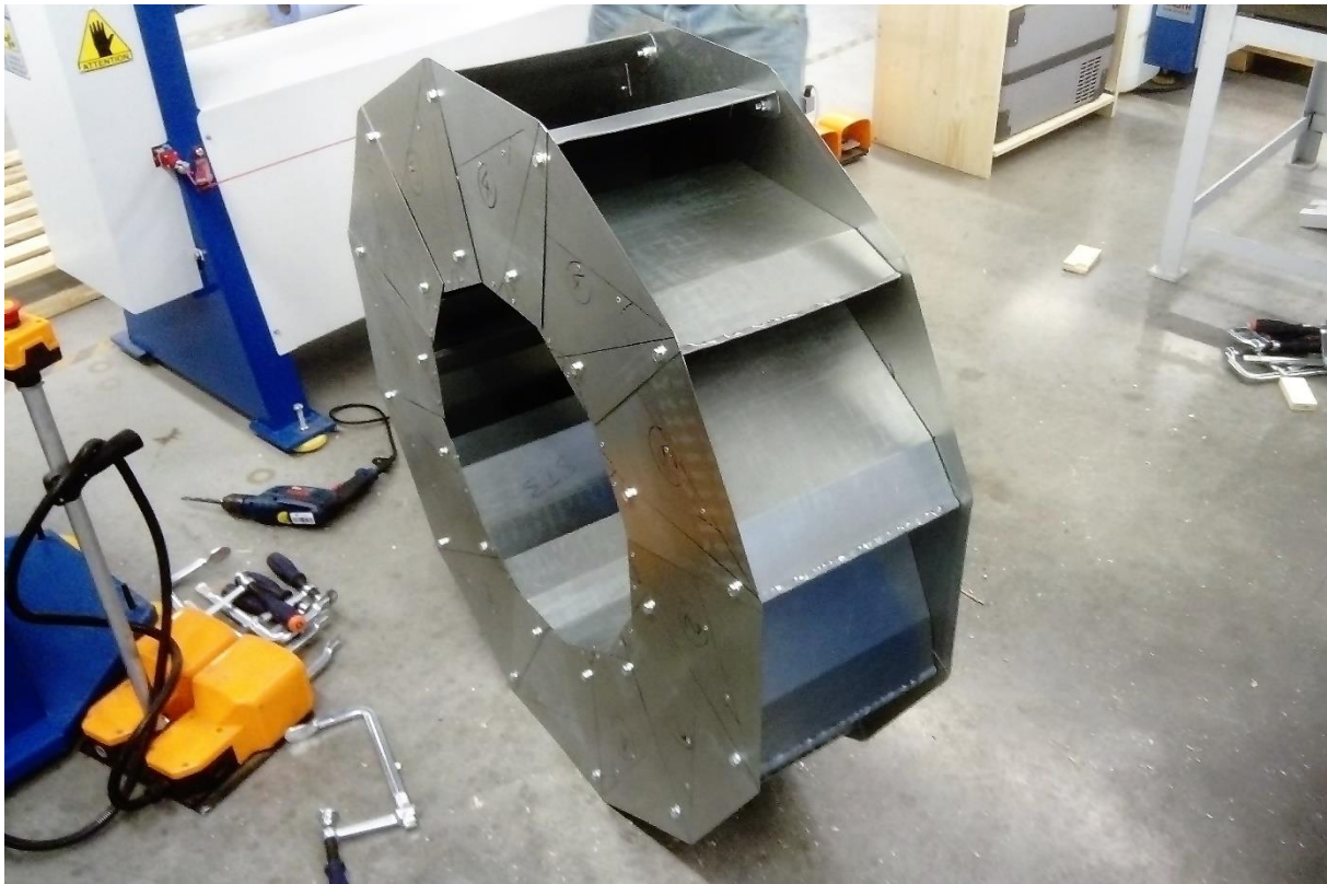
Figure 5-42: Finalized prototype rim – H = 1,3 \text{ m} ; Q = 0,02 \text{ m}^3/\text{s}
