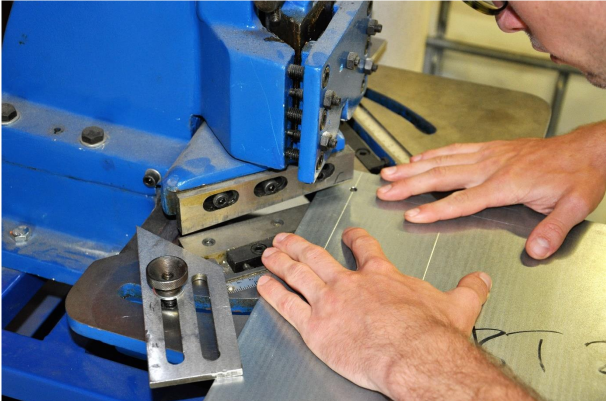
Figure 5-14: Notching the cornered cuttings
