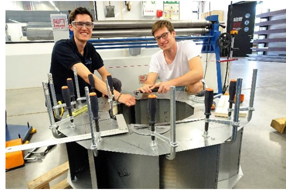
Figure 5-40: bolting the final shape of the water wheel
