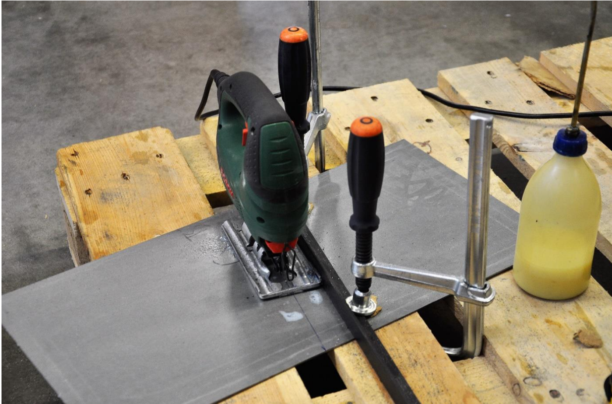
Figure 5-11: Use of a fence to guide the jigsaw
