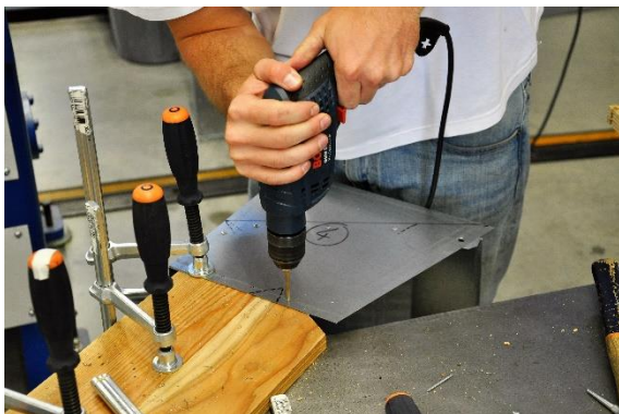
Figure 5-32: Processing the blind rivet holes in wall and bottom element
