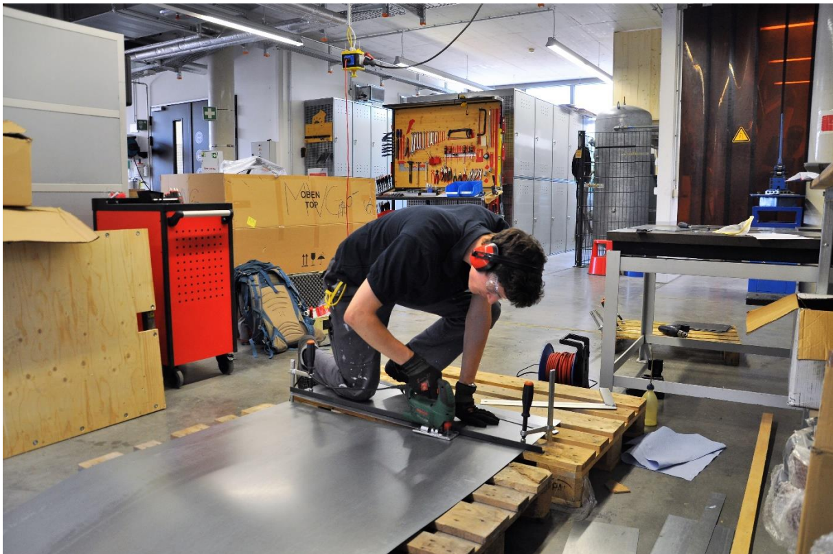
Figure 5-10: Basic cutting of the components from the raw sheet metal plate
