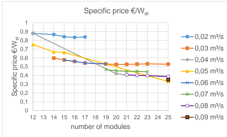
Figure 5-43: Specific price for the water wheel rim related to the electrical power output ( \text{€} / W_{el} )
