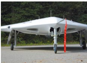
1 | SAGITTA multidisciplinary advanced research demonstrator – Flying Wing UAV.
