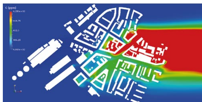
2 | Isosurface for CO 2 concentration of 425 ppm (left), surface concentration of CO 2 at z = 2m (right).
