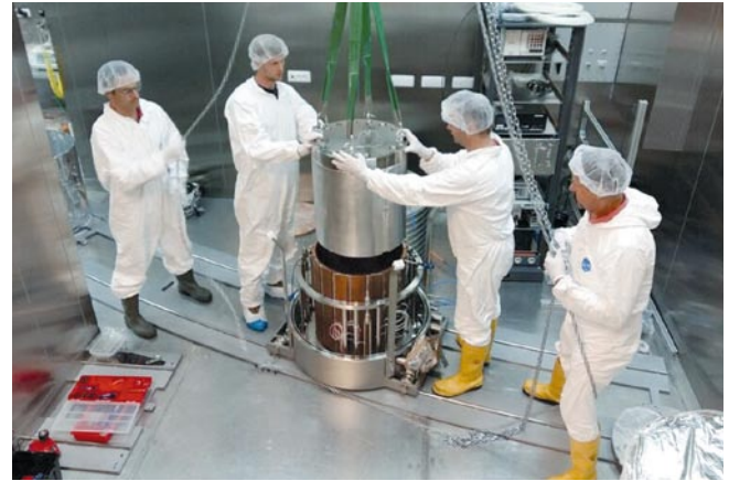
3 | Test-deployment of the TUM-Genova thermal calorimeter at the Laboratory Nazionali del Gran Sasso (Italy).
