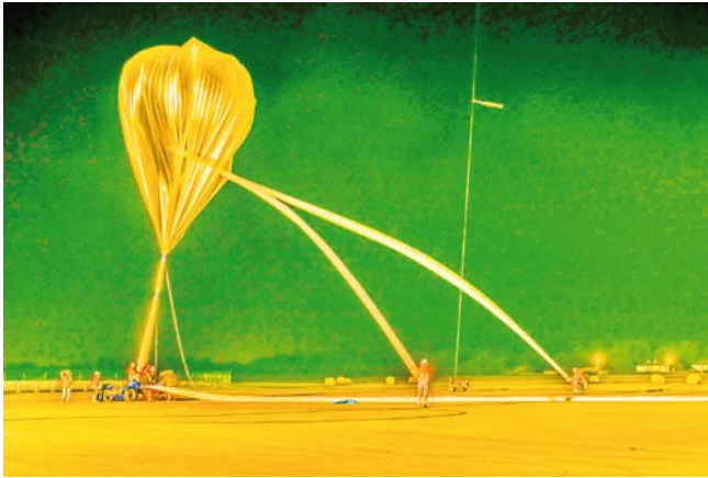
2 | Stratospheric balloon used for flying our prototype detectors, during its helium filling prior to the launch at Aire-sur-Adour (France) on July 2, 2016.
