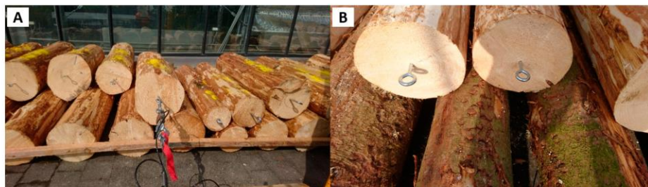
Figure 2. (A) Front display of the test setup and (B) open-eye hooks used for coupling to the measuring unit.
