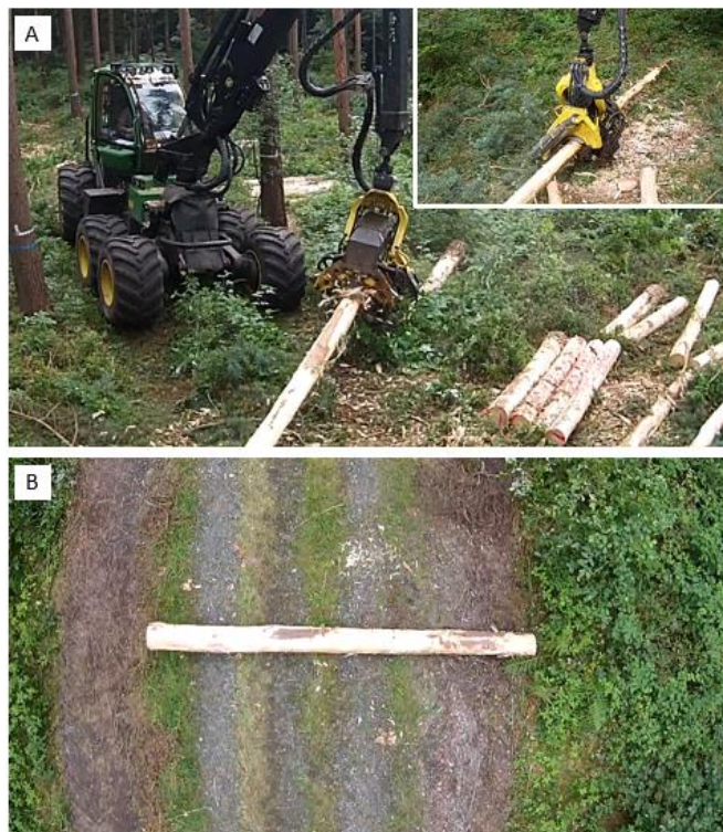
Figure 26: Footage recorded by a drone during the S1 summer field trials A) Debarking process of Scots pine, top and bottom view; B) Birdseye view of a debarked Scots pine log
