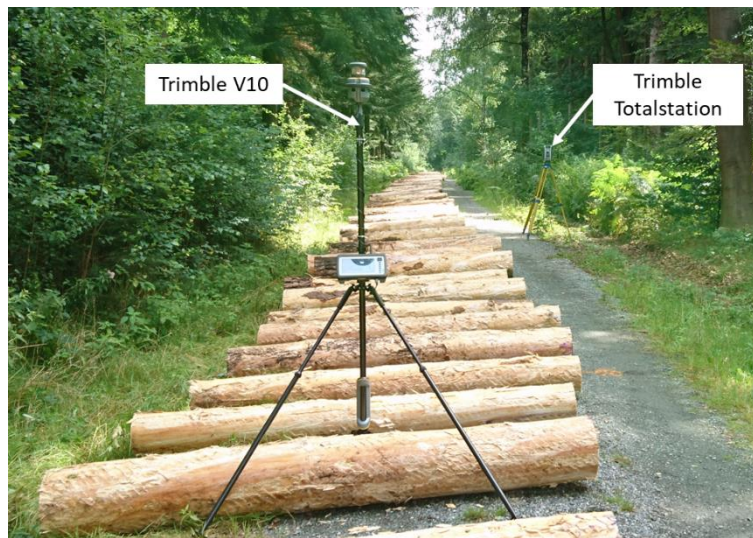
Figure 22: Measurement setup of a Trimble V10, connected to total station during the S1 Summer trials
