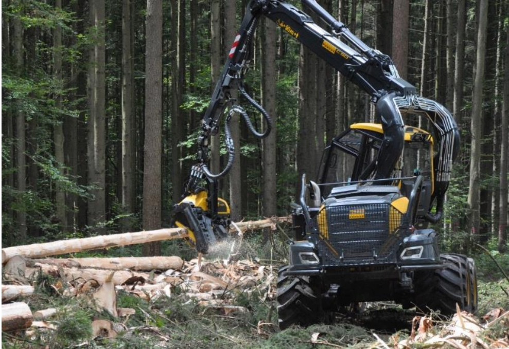
Figure 9: The S3 Setup in the Summer trial (Bavaria) on the third pass, cutting the stem into assortments after delimiting and debarking
