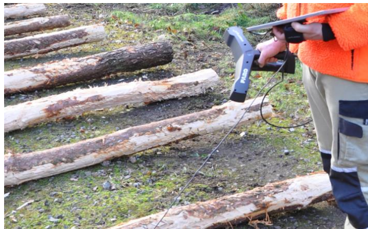
Figure 25: In field test applications of a Faro Freestyle3D laser scanner to record debarked Scots pine logs
