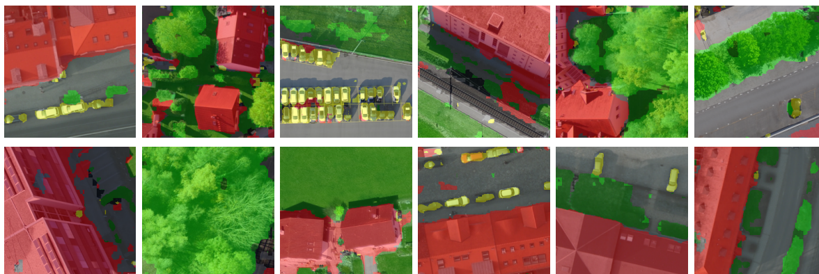
Figure 3. Example of semantic segmentation results on our validation images with a fine-tuned fully convolutional network (FCN) model [49] trained on UAV and aerial images. Visualization is color coded for buildings (■), streets (■), low vegetation (■), high vegetation (■), cars (■), and others (■).
