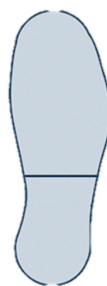
Figure 1. Detecting area division of the fore and rear foot part in loadsol force insole (adapted from [36]).
