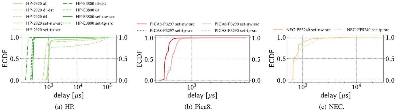
Fig. 3: Processing time of software rules for different vendors. Note that Dell does not support any software rules. We observe that software processing is much less predictable than hardware processing. Software processing is also orders of magnitude slower.
