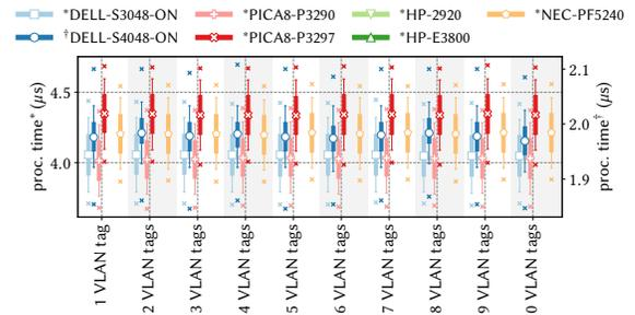
Fig. 15: Processing time of the different switches for matching on the outermost VLAN tag, popping it and forwarding to a particular queue based on different VLAN tag stacks heights. We observe that the switches can predictably support source routing solutions based on VLAN tags.
