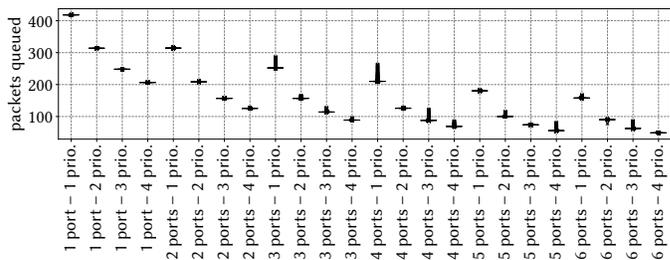
Fig. 12: Buffer capacity made available to a given queue of the Dell S3048-ON switch for different numbers of congested ports and queues (1516 bytes packets): the more ports and queues are overloaded, the less buffer is made available to a given queue.
