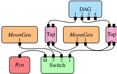
Fig. 4: Measurement setup for priority queuing investigation.
