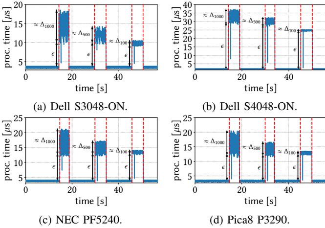
Fig. 5: Processing time of a high priority flow (bursts of 100 bytes packets) with 3 subsequent interfering low priority flows of, respectively, 1000, 500 and 100 bytes packets. We observe that the processing time increases more (by  $\epsilon$ ) than what network calculus predicts. We note that the behavior of Pica8 3297 switch is very similar to Pica8 3290 and hence not shown.
