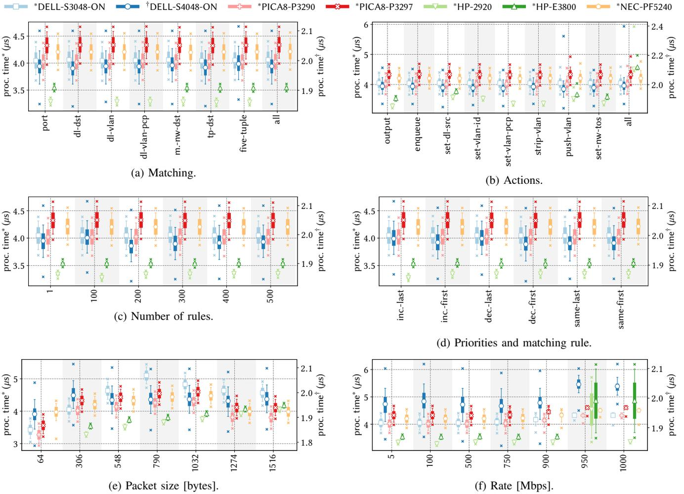
Fig. 2: Impact of the different considered dimensions on the hardware processing time of the different switches. The number of rules, their priority, the matching rule and its matching structure do not impact the processing time. The packet size is the main influential factor, while rate and action type impact only a subset of the investigated switches. Overall, the processing time of switches is predictable and can be deterministically bounded by a constant.
