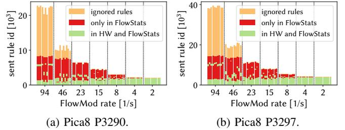
Fig. 8: Divergence of the flow table state of the Pica8 (a) P3290 and (b) P3297 switches for different *FlowModAdd* rates. For each rate, each stacked bar corresponds to a distinct run. Rules that are only in the *FlowStats* response of the switch are critical: while the controller thinks the packets will be forwarded, they will actually not be. The switch is then unpredictable.
