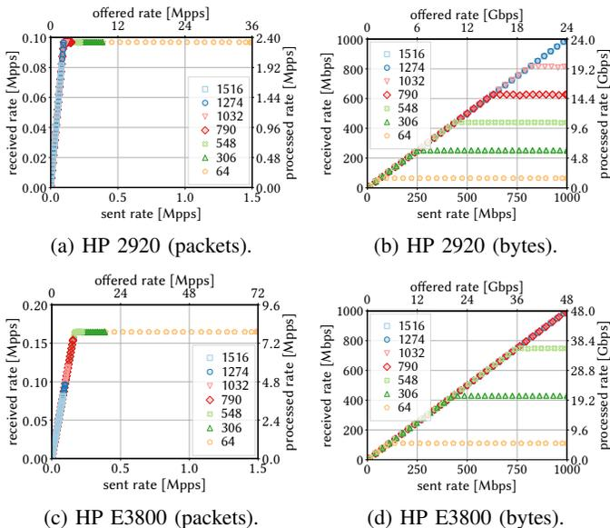
Fig. 7: Throughput of the HP switches. Lower (resp. left) axes correspond to the traffic sent (resp. received) on the first and last ports, i.e.,  $R_1^x$  and  $R_2^x$  (resp.  $R_1^y$  and  $R_2^y$ ). The upper (resp. right) axes correspond to the values scaled by the number  $n$  of ports to represent the total data rate actually processed by the switch.
