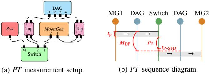
Fig. 1: (a) Switch processing time measurement setup and (b) corresponding sequence diagram.
