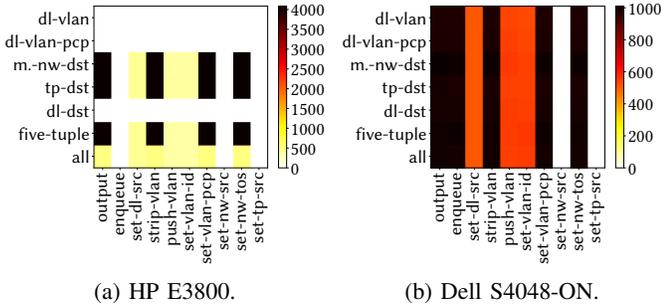
Fig. 10: Flow table size of the (a) HP E3800 and (b) Dell S4048-ON switches for the different match/action combinations. A size of 0 identifies a combination not supported in hardware. We observe that the table size depends on both the matching type and the action and can heavily influence the number of rules that can be inserted.
