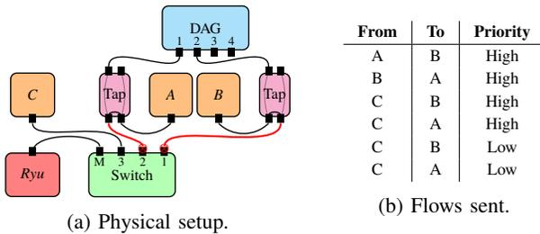
Fig. 11: Setup for evaluating buffer size with 2 congested ports and 2 congested queues per port. The congested ports are marked with a red cross.
