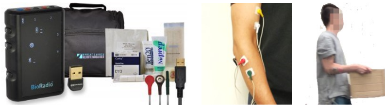
Figure 2: The sEMG sensors and the simulated material handling task
