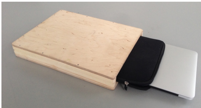
Figure 3-2: Self-made wooden hard case and inner soft sleeve for protecting the laptops from mechanical stress [Own Illustration]
