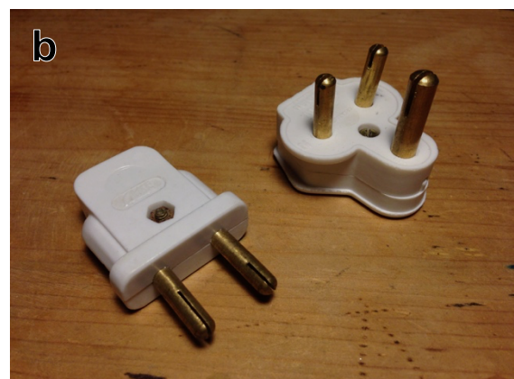
Figure 3-3: Nepali power socket (a) and Nepali type C (left) and type D (right) plugs (b) [Own Illustration]
