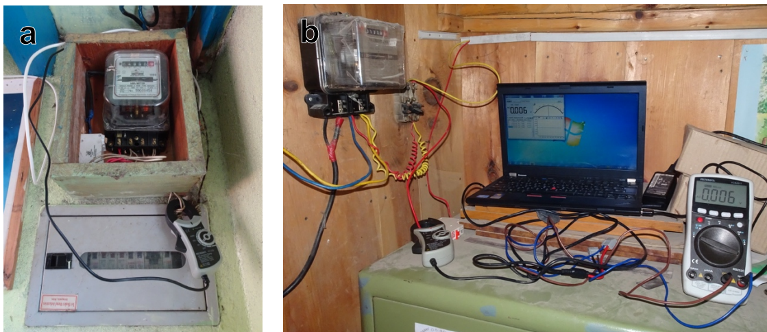
Figure 3-1: a: Main box with current clamp adapter enclosing the main wire of the single phased main box. b: Complete current measurement setup. [Own Illustration]
