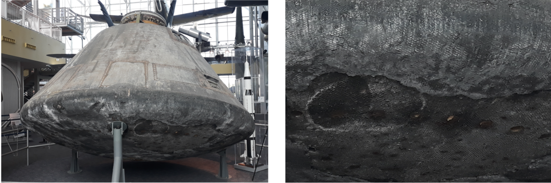
Figure 1.1: Photo of the Apollo 12 Command Module (left) and enlargement of the burnt TPS (right), taken at Virginia Air & Space Center, USA.
