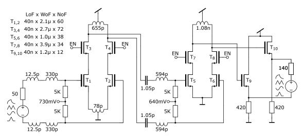
Figure A.4: Redesigned LNA operating in the frequency range 19 - 26 GHz taking into account resistive and capacitive interconnect parasitics.
