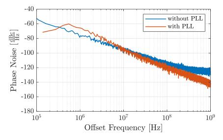
Figure 5.14: Phase Noise (PN) of the LO signal with and without the PLL. The carrier frequency is set in both cases to 10 GHz. The PN at the offset frequency around 10 MHz is almost equal for both cases. For the higher offset frequencies in case with the PLL the PN is improved.
