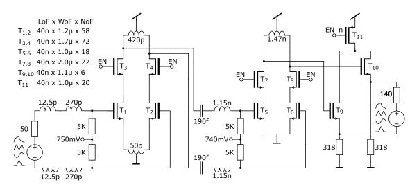
Figure A.6: LNA operating in the frequency range 33 – 39 GHz.
