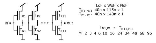
Figure A.12: Driver of the VCO depicted in Figure A.11. The eleven driver stages with increasing multiplier M is required to be able to drive the load at relatively high frequencies.
