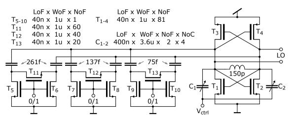
Figure A.13: VCO operating in the frequency range 19 - 26 GHz. The varactors  $C_{1-2}$  are build with NMOS capacitors.
