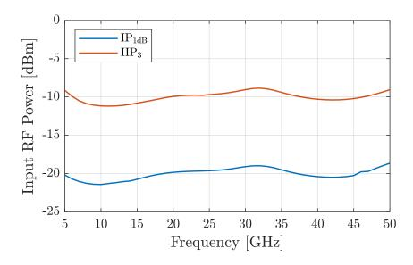
**Figure 5.8:** Input referred distortion parameters  $IP_{1dB}$  and  $IIP_3$  extracted at different operating frequencies. The values remain relatively stable. The typical 10 dBm difference between  $IP_{1dB}$  and  $IIP_3$  is apparent as well [119, p. 23].
