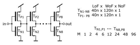
Figure A.10: Driver of the VCO depicted in Figure A.9. The finger dimensions of the NMOS and PMOS transistors are identical, except the multiplier M.
