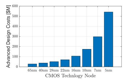
**Figure 1.1:** Rising design costs for the advanced technology nodes. Costs include Intellectual Property (IP) qualification, architecture, verification, physical and software design, prototype, validation. [1]
