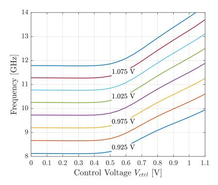
Figure 5.9: Frequency sweep of the VCO designed for 9-13 GHz and presented in Figure 4.11. The fine frequency tuning is achieved by the control voltage  $V_{ctrl}$ . The coarse frequency tuning is realized by sweeping the supply voltage of the inverter stages in steps of 25 mV.
