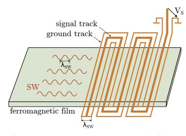
Figure 2.5: Coplanar waveguide as sensing element for SW detection propagating in a ferromagnetic thin film, e.g. YIG. The meander structure of the antenna improves the efficiency of the transduction [52]. The distance between two ground tracks of the waveguide should equal to the wavelength of the propagating SWs, in order to achieve high signal sensitivity (see also Figure 2.6).
