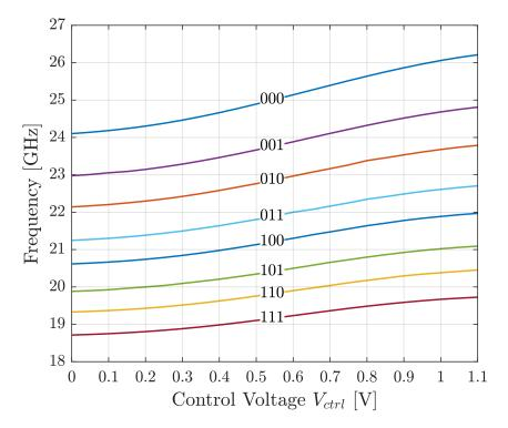
**Figure 5.12:** Adjustment of the VCO oscillating frequency in the range 19 – 26 GHz. The fine tuning of the frequency is made by the control voltage  $V_{ctrl}$  (see schematic in Figure 4.17). The coarse discrete tuning of the frequency is adjusted by digitally controlled input signals  $b_{0-2}$ .
