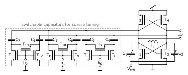
Figure 4.17: VCO designed to operate in the frequency range of 19 - 26 GHz. The topology is very similar to the schematic presented in Figure 4.14. Here, cross-coupled PMOS transistor are implemented, to set the common-mode voltage of the LO output nodes to the half of the supply voltage  $V_{dd}$  and consequently, to use the full control voltage range to adjust oscillating frequency [61, p. 530].
