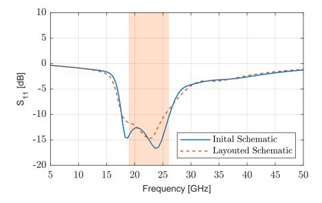
Figure 7.2: Pre- and post-layout simulation results of the input matching parameter  $S_{11}$ . The targeted performance below -10 GHz is almost achieved in the whole band of interest 19 - 26 GHz for both cases.
