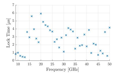
Figure 5.16: The simulated lock time of the PLL for integer oscillating frequencies of the LO signal. The tolerance of the control voltage is set to 5 mV, i.e. the variation of the control voltage is less than 5 mV after the lock time.
