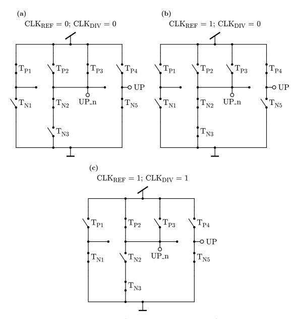
Figure 4.26: Demonstration of the operating principle of the PFD, presented in Figure 4.24. Three different states are considered, depending on the logical values of the reference clock  $CLK_{REF}$  and the divided LO signal  $CLK_{DIV}$ . The transistors are replace by ideal switches.
