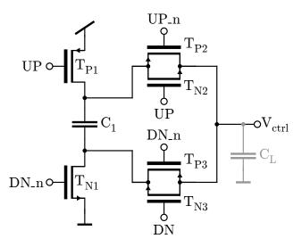
Figure 4.27: Charge Pump (CP) converting digital up and down pulses of the PFD (see Figure 4.24) into the analog control voltage  $V_{ctrl}$ . The charge transport from the supply to the output node is realized through the capacitor  $C_1$ . The gray marked capacitor  $C_L$  represents the load capacitance at the output node, resulted from the loop filter (see Section 4.6.4).
