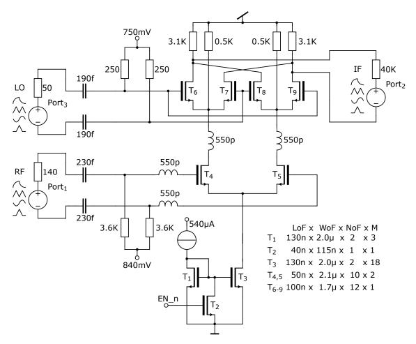
Figure A.8: Mixer operating in 9 - 50 GHz range.
