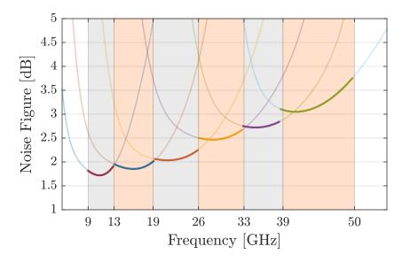
Figure 5.3: NF of the 6 LNAs operating at different frequency bands from 9 - 50 GHz. The minimum achievable NF is rising with increasing frequency due to the higher contribution of the transistors' gate resistances [71].
