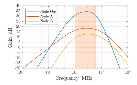
Figure 5.17: Gains of the OpAmp at nodes A, B and Out (see Topology in Figure 4.33). The band-pass characteristic of the second order is apparent. The reduction of the gain from node A to B is caused by the inter-stage buffer. In the desired frequency band 10-60 MHz the OpAmp achieves a gain higher than 30 dB.
