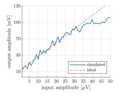
Figure 6.4: Amplitude change at the output of the SW readout circuitry due to the applied variation of the signal power at the input. The gain of the circuitry remains relatively linear till  $30 \,\mu\text{V}$ , as the comparison with the ideal curve shows.
