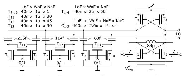
Figure A.14: VCO operating in the frequency range 26 - 33 GHz.
