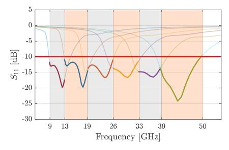
Figure 5.2: Scattering parameter  $S_{11}$  of the LNAs operating in 6 different frequency bands from 9 - 50 GHz. The red horizontal line corresponds to value of -10 dB, i.e. less than 10% of the LNA input signal is reflected back.
