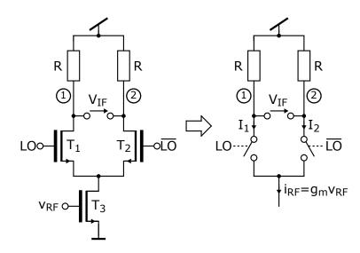
Figure 4.9: Simplified single-balanced mixer. Transistor  $T_1$  and  $T_2$  are replaced by two complementary switches. Transistor  $T_3$  generates a small signal current  $g_m v_{RF}$ . The output IF voltage results from the multiplication of the RF current and square wave switch functions.
