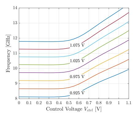
Figure B.1: Frequency tuning of the VCO designed for the frequency range 9 - 13 GHz.
