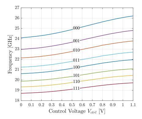
Figure B.3: Frequency tuning of the VCO designed for the frequency range 19 - 26 GHz.
