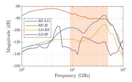
Figure 5.7: Characterization of the mixer's port isolation from RF to IF (RF-IF), from RF to LO (RF-LO), from LO to RF (LO-RF) and from LO to IF (LO-IF). A relatively low feedthroughs between all the port are achieved. The higher RF-IF feedthrough at lower frequencies is caused by amplified RF signal through transconductance transistors  $T_{4,5}$  (see Figure 4.8), that is easily filtered out by the following OpAmp.
