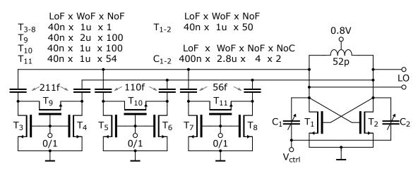
Figure A.16: VCO operating in the frequency range 39 - 50 GHz.
