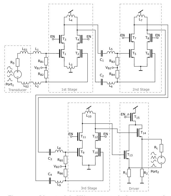
Figure 4.6: Schematic of the LNA operating in the frequency range of 39 - 50 GHz with the input signal picked up by an on-chip near field loop antenna. The LNA contains 3 amplifying stages in order to achieve a reasonable high voltage value for the RF input of the mixer (Port 2). Each stage consists of a cascode Common Source (CS) circuit with inductive loading. The first stage exhibits the inductive source degeneration  $L_3$  needed for the 50  $\Omega$  input matching.
