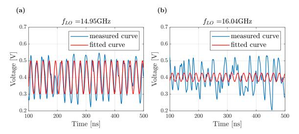
Figure 6.3: Transient simulation results for the readout circuitry outputs and its fitting curves resulted from post signal processing in MATLAB. Two frequencies of the LO signal 14.95 GHz (a) and 16.04 GHz (b) are considered. It demonstrates, that small frequency differences (10 - 60 MHz) between RF and LO signals can be recognized (a) by configured fitting tool. As targeted for larger frequency difference (b), the measured and the fitted curves do not match with each other.
