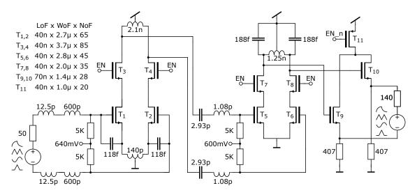
Figure A.1: LNA operating in the frequency range 9 - 13 GHz.
