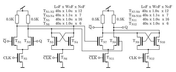
**Figure A.18:** SFD divider with dividing factor 2 operating till 40 GHz. The outputs Q and  $\overline{Q}$  of the second flipflop are connected to the inputs of the first flipflop.
