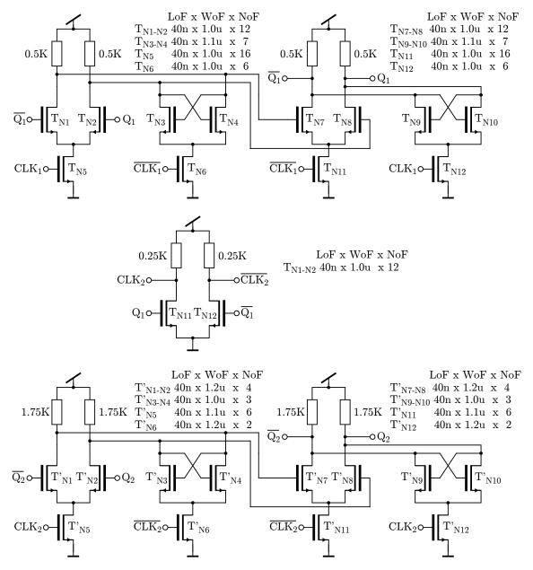
**Figure A.20:** SFD divider with dividing factor 4 operating till 40 GHz. The outputs  $Q_{1/2}$  and  $\overline{Q_{1/2}}$  of the second flipflops are connected to the inputs of the first flipflops. Inter-stage buffer recovers the divided clock signal CLK<sub>1</sub> and provides the clock signals CLK<sub>2</sub> and  $\overline{\text{CLK}}_2$  for the second divider.
