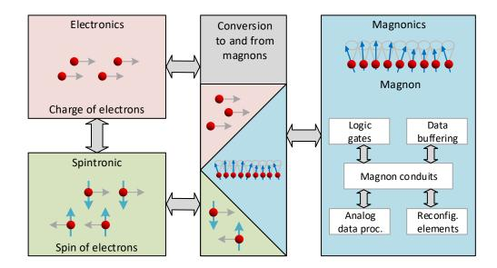
Figure 1.2: Schematical overview of the conversion between electronics, spintronics and magnonics with charge of electrons, spin of electrons and magnon, accordingly, as quanta for information processing. The electronic domain is used to control transducers converting the signal into the magnonic domain, where information is processed in an energy efficient way and is finally converted back into the electronic domain. Figure is adopted from [13, Figure 1].
