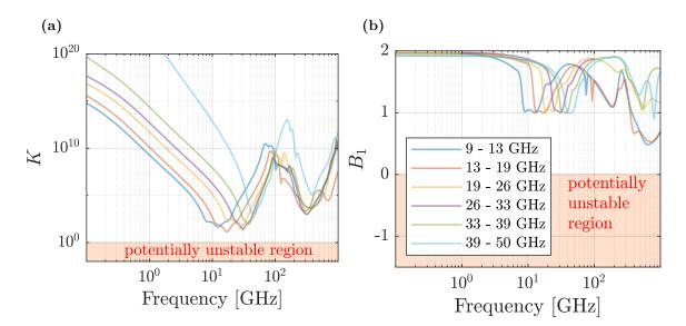
Figure 5.4: Stability parameters K (a) and  $B_1$  (b). Parameters extracted from the simulation results of the LNAs operating in 6 different frequency bands. Legend in (b) also applies for (a). For *unconditional stability* the inequalities K > 1 and  $B_1 > 0$  have to be hold.
