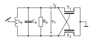
Figure 4.16: LC oscillator with equivalent parasitic resistance  $R_p$  at the resonance frequency. The cross-coupled transistors  $T_{1-2}$  generate a negative resistance in order to cancel out the lossy part of the tank.
