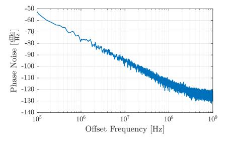
Figure 5.13: Phase Noise (PN) of the VCO operating in 9-13 GHz. The carrier frequency is set to the maximum adjustable values, i.e. the control voltage  $V_{ctrl}$  and the supply voltage  $V_{sup}$  are set to 1.1 V (see schematic in Figure 4.11).
