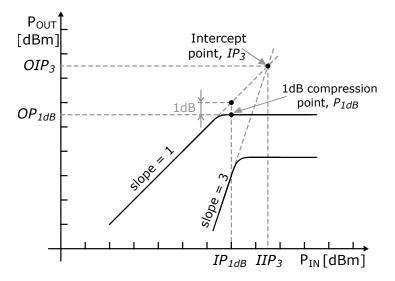
Figure 3.5: Definitions of the linear distortion parameters the 1 dB compression point  $P_{1dB}$  and the 3rd order intercept point  $IP_3$ . The curves represent the 1st and the 3rd order intermodulation products of the output power versus the input power in a log-log scale. Both responses indicate a compression at a certain input power. The ideal responses are extended with dashed lines.
