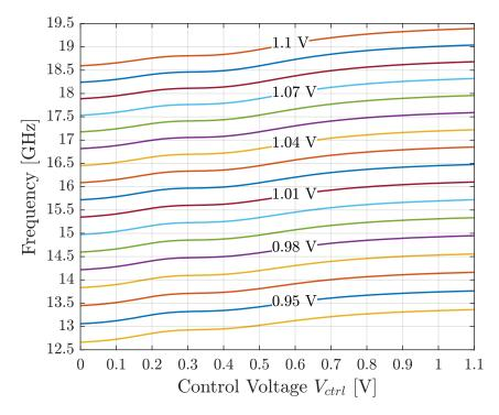
**Figure B.2:** Frequency tuning of the VCO designed for the frequency range 13 - 19 GHz.
