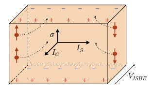
Figure 2.4: Sketch of the working principle of the Inverse Spin Hall Effect (ISHE). The spin current  $I_S$  with the spin polarization  $\sigma$  results in the electrical charge current  $I_C$  and the ISHE voltage  $V_{ISHE}$  [49].
