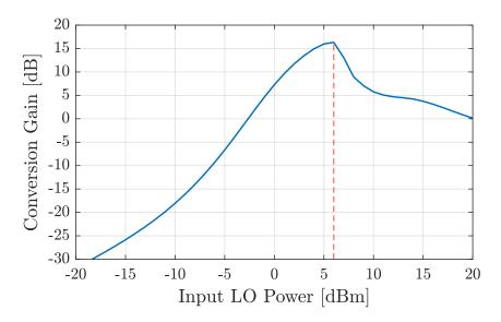
Figure 5.5: Conversion gain of the mixer versus input LO power. For this simulation the frequencies of the RF and LO signals are set to 25.02 GHz and 25 GHz, respectively. The maximum value of the conversion gain is achieved at 6 dBm.
