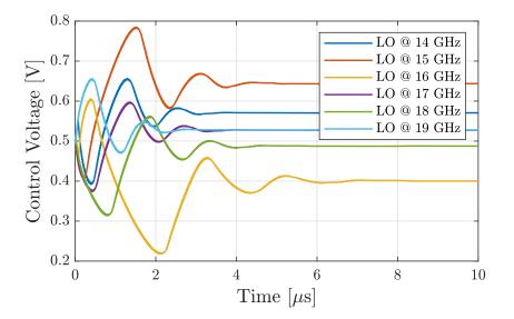
Figure 5.15: The transient simulation results of the VCO control voltage at different frequencies. Figure demonstrates the locking behaviour of the PLL. The reference frequency of the PLL is applied in way, in order to get the integer oscillating frequencies between 14 and 19 GHz of the LO signal.
