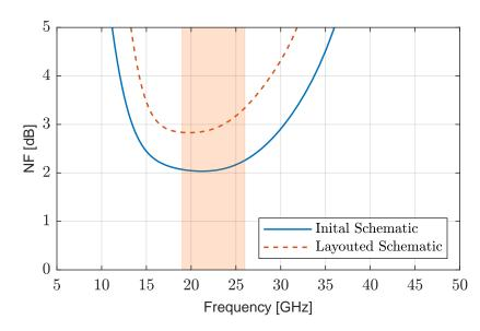
Figure 7.3: Noise Figure (NF) degradation of the LNA due to extracted interconnect parasitics resulted from the layout. The simulation results show 1 dB higher NF for the extracted schematic.
