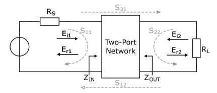
Figure 3.2: Illustration of the S-parameter definitions of a two-port network with source resistance  $R_S$  and load resistance  $R_L$ .  $E_i$  and  $E_r$  denote incident and reflected waves, respectively.  $Z_{IN}$  and  $Z_{OUT}$  represent input and output impedances of the two-port network.
