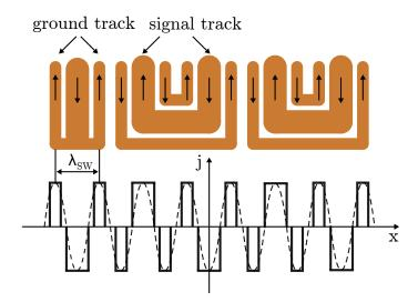
Figure 2.6: Spatial distribution of the current density flowing through the coplanar waveguide. The geometry of the waveguide is selected with the target for achieving a close approximation to a sinusoidal distribution as close as possible. Figure is adopted from [52].
