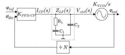
Figure 4.31: Block diagram of the PLL with its transfer functions. The PFD and the CP are combined to one block, due to a representation by a single transfer function. The loop filter is described by the impedance  $Z_{LF}$ .
