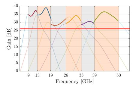
Figure 5.1: Voltage gain of the LNAs operating in 6 different frequency bands from 9-50 GHz. The values at the abscissa correspond to limits of the bandwidths, that marked with alternating colors. The red horizontal line is sketched at 26 dB and shows that all LNAs achieve the amplification factor of at least 200.
