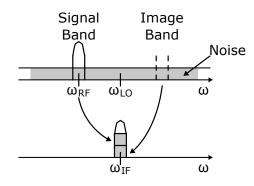
Figure 3.4: Noise contribution from the signal band and the image band to the total noise at the IF output of the mixer. By down-converting the RF signal to the lower IF signal, the additional undesired noise at  $\omega_{LO} + (\omega_{LO} - \omega_{RF})$  is added to the noise from the signal band at  $\omega_{LO} - \omega_{RF}$ .
