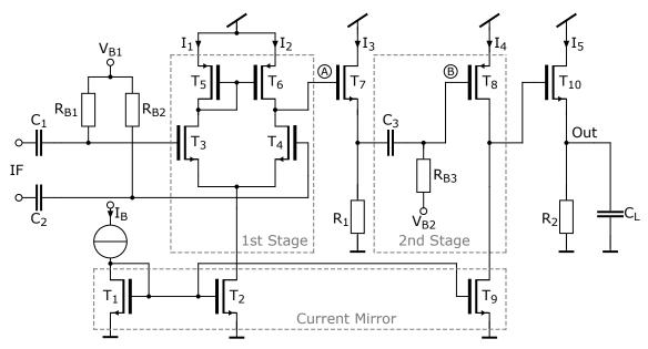
Figure 4.33: Topology of the differential single-ended Operational Amplifier (OpAmp) with two amplifying stages. Each stage is followed by a buffer to drive the high capacitive load. The DC current to the stages is provided by  $I_B$ . The DC gate voltages of the transistors  $T_{3-4}$  and  $T_8$  are adjusted by bias voltage source  $V_{B1}$  and  $V_{B2}$ , respectively.
