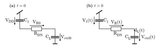
Figure 4.30: Simplified representation of the CP circuitry in the pump down mode. The resistor  $R_{DN}$  models the on-resistance of the closed transmission gate switch  $T_{N3,P3}$  (see Figure 4.28b). The initial voltages across the electronic components at the beginning of the pump down mode (t = 0) are presented in (a). Figure (b) demonstrates the definitions for the time dependent voltages and currents.
