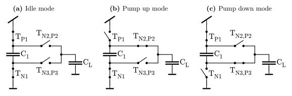
Figure 4.28: Operating modes of the CP. The idle mode (a) is required for pre-charging the capacitor  $C_1$ . The pump up (b) and down (c) modes are for increasing and decreasing the control voltage at the output node, respectively.
