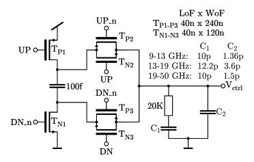
**Figure A.23:** Charge Pump (CP) with LF. For the NMOS transistors minimal sizes of the gate length and width are used. Depending on the VCO operating frequency, the filter capacitances  $C_1$  and  $C_2$  are adjusted due to stability reasons.
