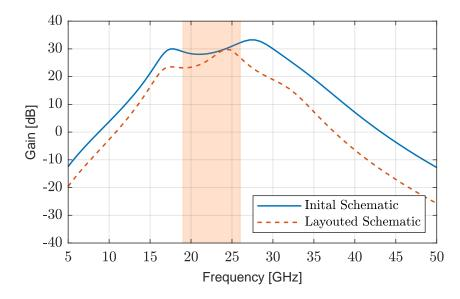
Figure 7.1: Voltage gain of the LNAs designed for the frequency range 19 - 26 GHz. The curve in blue shows the gain performance of the initial design. The redesigned version considering interconnect parasitics is depicted in the dashed curve.
