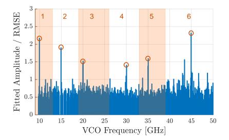
Figure 6.2: Simulation results for the SW frequency measurement. The output of the VCO signal, LO, is swept between 9-50 GHz with steps around 20 MHz. The maxima in each of the 6 frequency bands correspond to the applied frequencies of the input signals assumed in the loop antenna.
