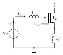
Figure 4.5: CS circuit with parasitic gate-source-capacitance, degenerating inductor  $L_3$  and serial inductor  $L_1$  for canceling the reactive component of the small signal input impedance  $z_{in}$ .
