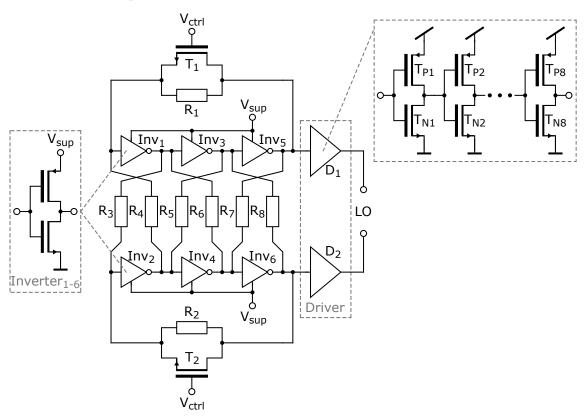
Figure 4.11: VCO operating in frequency range of 9-13 GHz. The schematic includes the differential ring oscillator with three stages, the delay element in the feedback path, phase balancer resistors between two ring oscillators and the drivers at the output decoupling the oscillator from the load capacitance of the followed circuitry.
