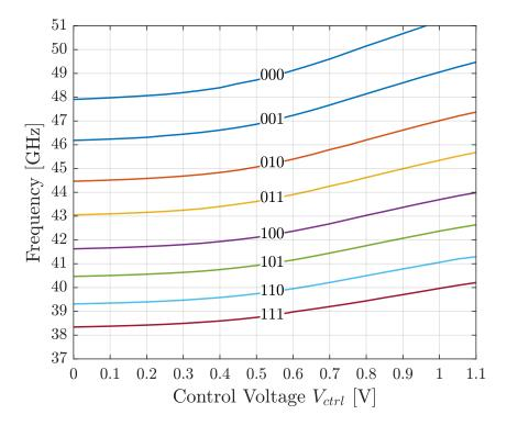
Figure B.6: Frequency tuning of the VCO designed for the frequency range 39 - 50 GHz.
