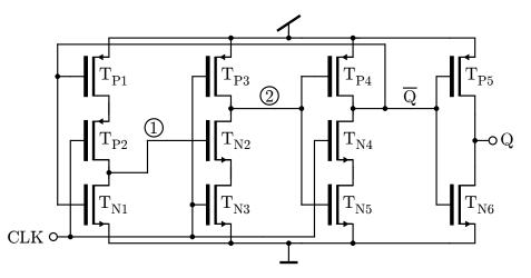
Figure 4.19: True Single-Phase Clocking (TSPC) frequency divider. The input clock signal CLK propagates to the output Q resulting in the frequency division by factor 2. The dynamic logic technique is used to achieve high frequency operations till 18 GHz.
