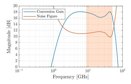
Figure 5.6: Conversion gain and NF of the designed mixer (see Figure 4.8). In the marked bandwidth of interest 9 - 50 GHz the voltage conversion gain is more than 16 dB and the NF less than 12 dB.
