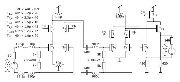
Figure A.5: LNA operating in the frequency range 26 - 33 GHz.
