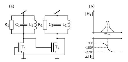
Figure 4.15: Simplified version of the LC oscillator (a) and the sketched gain and phase of the transfer function for the first stage. The cross-coupled transistors can be considers as two amplifying stages with a feedback loop.  $R_1$  and  $R_2$ represent equivalent parallel resistances at the resonant frequency  $\omega_{osc}$  of the LC tanks. The required 180° phase shift per stage occurs at the resonance frequency  $\omega_{osc}$ . [61, pp. 512-513]
