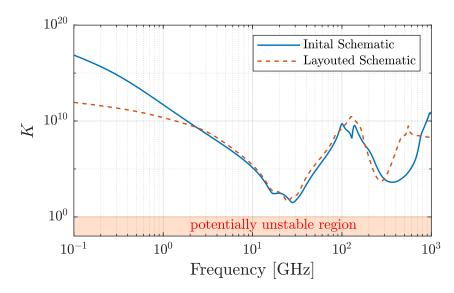
Figure 7.4: Stability factor K of the pre- and post-layout schematic. The simulation results show, the LNA still remains stable after the redesign.
