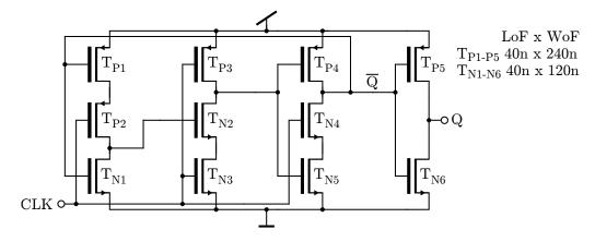
Figure A.17: TSPC divider operating till 18 GHz. Minimum sized NMOS and PMOS transistors are used.
