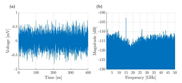
Figure 6.1: Voltage signal of the SW transducer model in time (a) and frequency (b) domain. The applied frequency is equal to 15 GHz. The amplitude is set to  $10 \,\mu\text{V}$ . The thermal noise results in from the 50  $\Omega$  resistance of the loop antenna (see Section 2.3).
