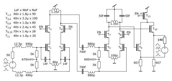
Figure A.2: LNA operating in the frequency range 13 - 19 GHz.
