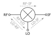
**Figure 3.6:** Port-to-port feedthroughs of a mixer with Radio Frequency (RF), Local Oscillator (LO) and Intermediate Frequency (IF) ports. The coupling between the ports is caused by parasitic capacitances of the used electronic devices.
