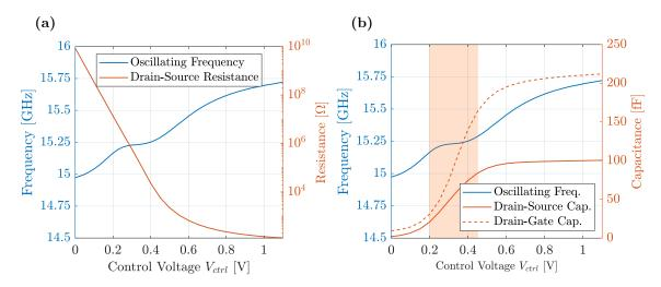
Figure 5.11: Frequency sweep of the VCO designed for 13 - 19 GHz. The selected curve for the oscillating frequency is for the supply voltage of 1 V. The red curves show the output resistance a) and the drain capacitances b) of the control transistor T<sub>C</sub> (see Figure 4.13) for the fine frequency tuning.
