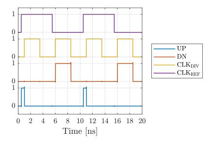
Figure 4.25: Input and output signal of the PFD (see schematic in Figure 4.24). If at the rising edge of  $CLK_{DIV}$  there is a difference to the reference clock, then the down pulse DN is generated. Equivalently, the up pulse UP is generated at the rising edge of the reference signal  $CLK_{REF}$ .
