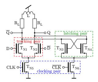
Figure 4.23: D-latch of the SFD operating till 50 GHz. The inductive loading is introduced to compensate for the capacitances at the output nodes Q and  $\overline{Q}$ . The whole circuitry of the SFD with parameter values of the electronic devices is attached in Appendix Figure A.21.
