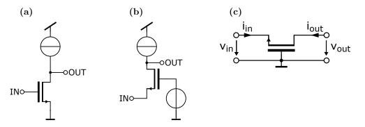
**Figure 4.2:** (a)Common Source (CS), (b) Common Gate (CG) and (c) the equivalent small signal circuit of the CG. In RF and mmW design the CS is used for a lower NF. For better input matching the CG is a better choice.
