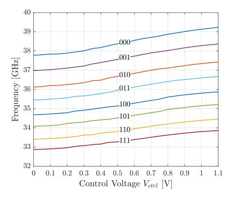
Figure B.5: Frequency tuning of the VCO designed for the frequency range 33 - 39 GHz.
