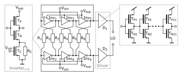
Figure 4.13: VCO operating in the frequency range 13 - 19 GHz. The topology is very similar to the design depicted in Figure 4.11. The difference is in the implementation of the delay element for frequency fine tuning, in order to achieve higher operating frequencies. Besides, the number of inverter stages in the drivers are higher for the same reason.
