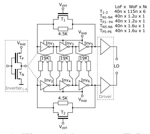
Figure A.9: VCO operating in the frequency range 9 - 13 GHz.  $T_N$  and  $T_P$  symbolize NMOS and PMOS transistors, respectively.
