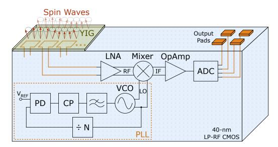
**Figure 4.1:** Concept of the SW detection with on-chip near field antennas placed below Yttrium-Iron-Garnet (YIG). The picked up signal is amplified and converted to lower frequencies with a circuitry realized in 40 nm CMOS technology. The digital information on the SW frequency, amplitude change and phase shift can be analyzed at the output pads.
