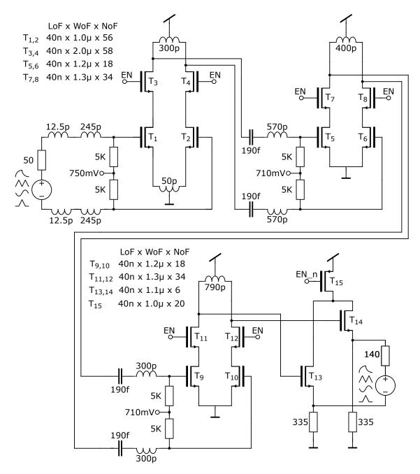
Figure A.7: LNA operating in the frequency range 39 - 50 GHz.
