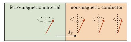
Figure 2.3: Spin Pumping (SP) effect by contacting the magnetic material with a non-magnetic metallic conductor. The magnetization dynamics in magnetic materials result in the spin current  $I_S$  flowing into the adjacent conductor.
