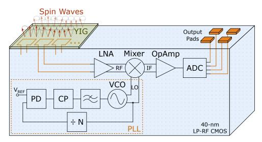
Figure 1.3: Conceptual schematic of Spin Wave (SW) on-chip detection. The SWs, propagating in the YIG film, are picked up with near field on-chip antennas. The transduced signal is processed in a CMOS Integrated Circuit (IC) (see Chapter 4). Information about SW frequency, amplitude change or phase difference between two SW signals is provided at the output pads in a digital form.
