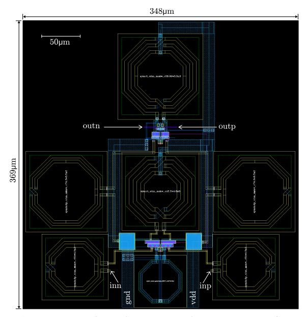
Figure 7.6: Layout of the LNA operating in the frequency range 19 - 26 GHz. The negative and positive inputs are marked with *inn* and *inp*, respectively. Similarly, it is applied for the output of the LNA. The positive and negative supply voltage is indicated by *vdd* and *gnd*, respectively. The schematic of the circuitry with electronic device dimensions can be found in Figure A.4.
