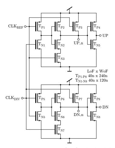
**Figure A.22:** Phase Frequency Detector (PFD) realized with dynamic logic. For the NMOS transistors minimal sizes of the gate length and width are used. The PMOS transistors have doubled gate width to have similar rising and falling time of the circuitry.
