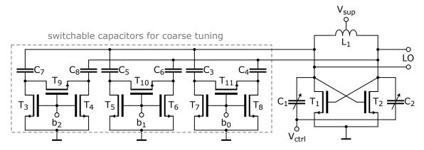
Figure 4.14: VCO operating in the frequency range 39 - 50 GHz. The inductor and the capacitors at the LO output nodes build the core of the circuit. Crossed-coupled transistors generate a negative resistance to cancel out parasitic resistance of the LC block. Fine tuning of the frequency is made by control voltage  $V_{ctrl}$ . The coarse frequency tuning is adjusted by binary coded switches  $b_{0-2}$ .
