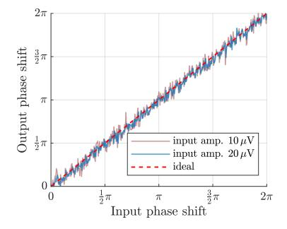
Figure 6.5: Phase shift measurement with the SW readout circuitry for two different input amplitudes  $10 \,\mu\text{V}$  and  $20 \,\mu\text{V}$ . The y-axes shows the phase shift considered at the output of the circuitry by applying a phase shift in the readout antenna. Comparison with the ideal curve reveals the deviation of the simulated results cause by the noise.
