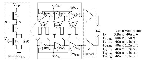
Figure A.11: VCO operating in the frequency range 13 - 19 GHz.  $T_N$  and  $T_P$  symbolize NMOS and PMOS transistors, respectively.
