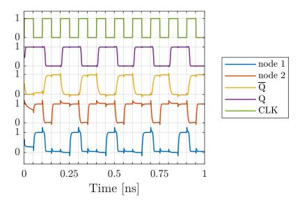
Figure 4.20: Transient simulation results of the TSPC divider with assumed clock frequency of 10 GHz. The voltage levels of the input and output nodes as well as the inter-stage nodes are normalized to the logical values 0 and 1. The observable small picks in the inter-stage node signals result from the parasitic capacitive coupling between the input and output of the respective stage.
