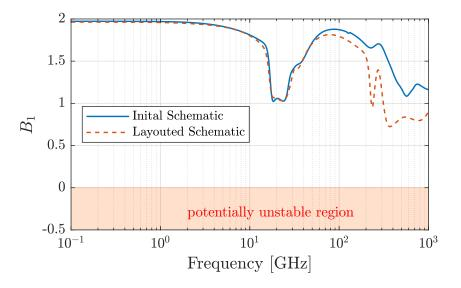
Figure 7.5: Stability factor  $B_1$ . The curves for both initial and layouted schematic are in the stable region.
