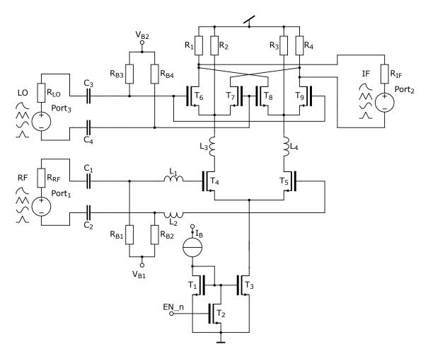
Figure 4.8: Topology of the double balanced Gilbert cell mixer, operating in the frequency range 9 - 50 GHz. The Radio Frequency (RF) signal is down-converted to the Intermediate Frequency (IF) signal by multiplication with the Local Oscillator (LO) signal. The topology is extended with inductors to achieve a better conversion gain and NF performance at around 30 - 50 GHz.
