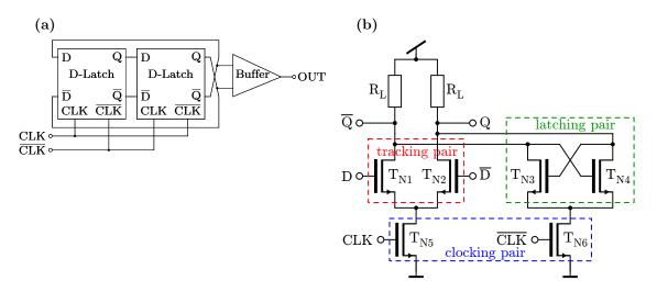
Figure 4.21: Static Frequency Divider (SFD) by factor 2 designed for the frequency range 18 - 40 GHz. The divider is realized by two alternated clocked D-latches (a). The transistor level schematic of the D-latch (b) contains the tracking, latching and clocking transistor pairs. The dimensions of the electronic devices are provided in Appendix Figure A.18.
