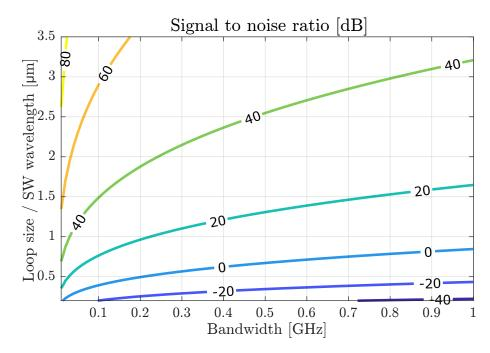
Figure 2.8: Simulated Signal-to-Noise Ration (SNR) of the squared loop antenna depending on its size and the considered bandwidth. The ordinate of the graph is normalized to the wavelength of the SW. As to expect, a larger area and a smaller bandwidth show a better SNR. [134]
