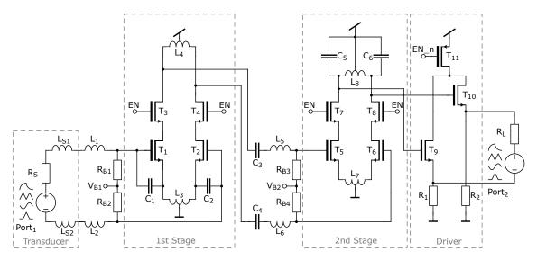
**Figure 4.3:** Topology of the LNA operating in the frequency range of 9 - 13 GHz. The differential transducer signal is amplified in two stages, which is capacitively coupled with  $C_{3,4}$ . Each stage is implemented with a common-source and cascode circuitry. The load impedance of the LNA is driven by source followers. EN symbolizes *enable* signal, switching between ground 0V and supply voltage 1.1V.
