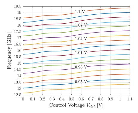
Figure 5.10: Frequency sweep of the VCO designed for 13-19 GHz. Schematic of the circuit is presented in Figure 4.13. The fine frequency tuning is adjusted by the control voltage  $V_{ctrl}$ . The coarse frequency tuning is realized by sweeping the supply voltage of the inverter stages in steps of 15 mV.
