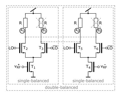
Figure 4.7: Topology of the double-balanced mixer as a combination of two single-balanced variants. The small signal voltage  $v_{RF}^+$  is equal to the negative voltage of  $v_{RF}^-$ . Consequently, for the double-balance configuration nodes  $A_1$  can be connected with  $B_2$  and  $B_1$  with  $A_1$ . LO and  $\overline{\text{LO}}$  represent complementary Local Oscillator (LO) signals.
