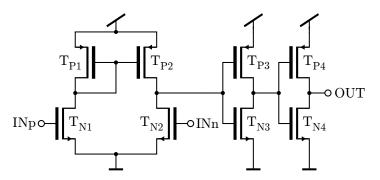
**Figure 4.22:** SFD divider buffer from the block diagram in Figure 4.21a. The circuitry includes differential comparator followed by two inverter stages. The dimensions of the circuitry are shown in Appendix Figure A.19.
