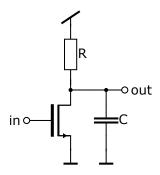
Figure 4.12: Simplified model of the inverter stage at the beginning of the oscillation. The input and the output are considered as small signal voltages.
