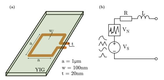
Figure 2.7: Sketch of the loop antenna placed below the non-conductive material YIG (a) and its equivalent circuit model (b). The squared loop antenna has the side length a, width of the wire w and thickness of the wire t. The resistance R and the inductance L result in from the geometry of the transducer. In addition, the model includes the voltage source  $V_S$  with the noise source  $V_N$ , originated mainly from the thermal noise of the conductor.
