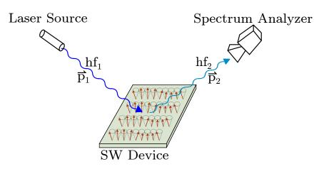
Figure 2.2: The principle of the BLS measurement technique for SW characterization. The frequency difference of the incident and scattered waves is used to analyze the SWs propagation in a sample. The spectrum analysis of the reflected electro-magnetic wave is performed with a Fabry–Pérot interferometer [33].
