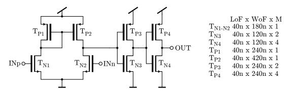
Figure A.19: Output buffer of the SFD divider.
