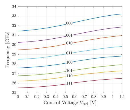
**Figure B.4:** Frequency tuning of the VCO designed for the frequency range 26 - 33 GHz.
