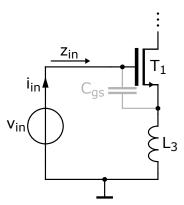
Figure 4.4: CS circuit with parasitic gate-source-capacitance and degenerating inductor. Small letters used for the input parameters mean small signal consideration.
