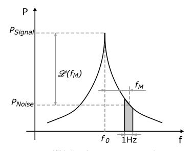
**Figure 3.7:** Phase noise  $\mathscr{L}(f_M)$  defined by the ratio of the noise power  $P_{Noise}$  at the frequency  $f_0 + f_M$  to the signal power  $P_{Signal}$  at the frequency  $f_0$ . The power is calculated for a frequency band of 1 Hz.
