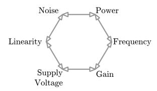
Figure 3.1: RF design hexagon representing trade-offs between parameters, e.g. the smaller the influence of the noise and the wider the operating frequency band, the more power is consumed by the circuit. [61, p. 4]
