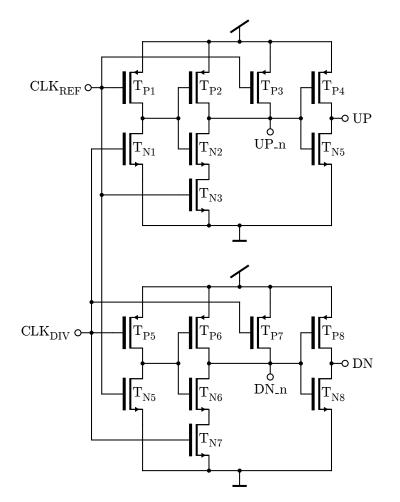
Figure 4.24: Topology of the implemented Phase Frequency Detector (PFD) operating in dynamic logic. Depending on the difference of the divided LO signal  $CLK_{DIV}$  and the reference clock  $CLK_{REF}$ , the up and down pulses at the output are created to adjust the phase and the frequency of the VCO.
