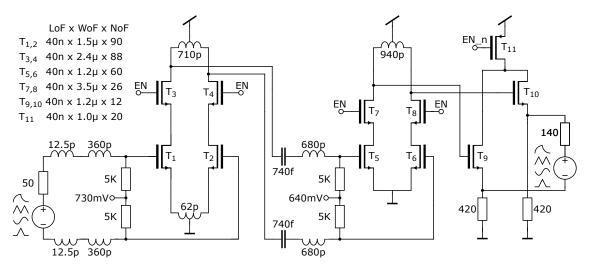
Figure A.3: LNA operating in the frequency range 19 - 26 GHz.
