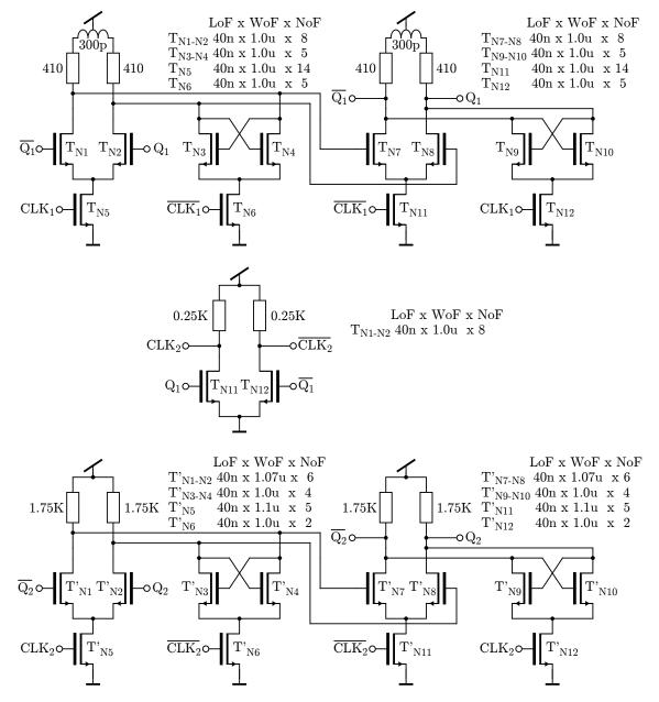
**Figure A.21:** SFD divider with dividing factor 4 operating till 50 GHz. The operation principle is similar to the topology depicted in Figure A.20. To achieve functionality above 40 GHz the inductive peaking technique is used in the first flipflop.
