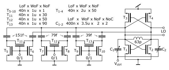
Figure A.15: VCO operating in the frequency range 33 - 39 GHz.
