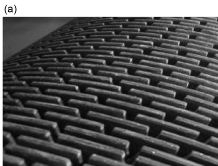
Fig. 2 – Cutting head and typical surface texture. (a) Grinding head. (b) Typical diamond ground texture.
