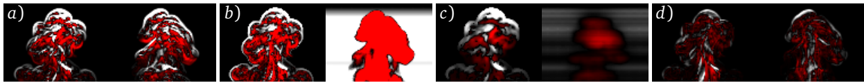
Figure 4.10.: Front and side views of 3D density changes. The ground truth density change leading from one time step to another is shown in a). Estimating the density of the next time via traditional tomography results in a density field uniformly distributed along each line of sight. By building the difference to the current ground truth density field, we obtain the density change shown in b). First calculating the difference in 2D image space and then projecting it into 3D space plus using a smoothness prior, leads to the density change in c). Our calculated density change is shown in d). While the front views match the ground truth density change well, our method overall obtains the most plausible and natural density changes as observed in the side views. Our density values are slightly too small but match the ground truth density change well.
