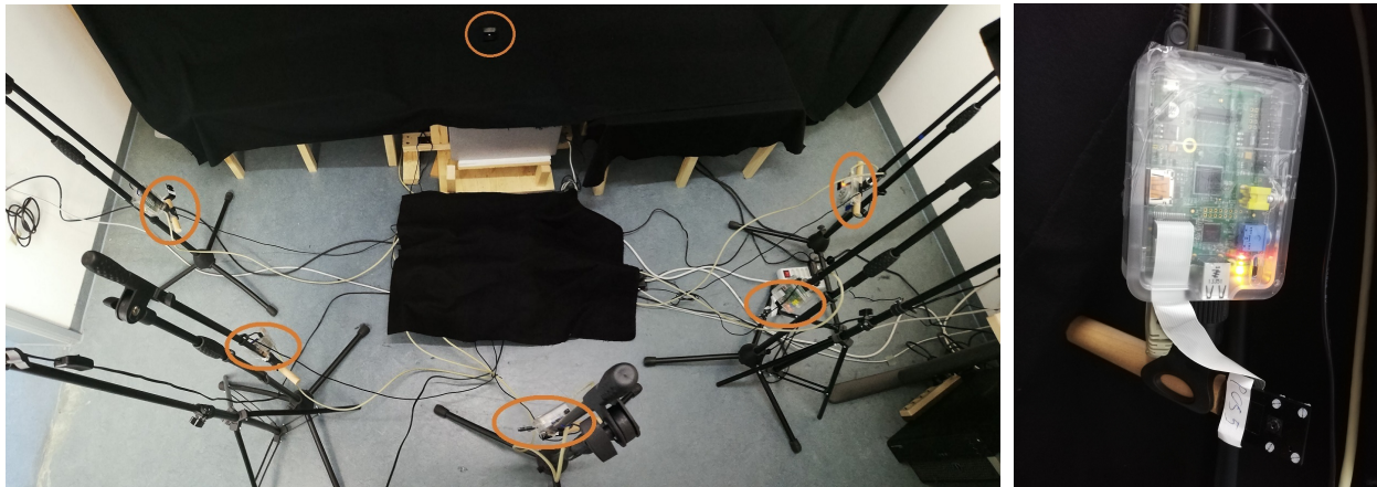
(a) Top-down view of microphone stands with cameras focusing on the smoke release, where both cameras and smoke release are marked by orange circles. (b) Close-up of Raspberry Pi computer with mounted camera module.
