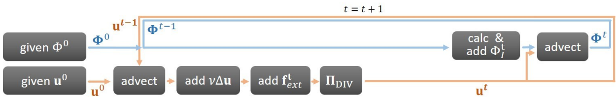
Figure 3.1.: Steps of a typical forward fluid simulator calculating velocity \mathbf{u}^t and density \Phi^t . The steps for velocity are denoted with orange arrows while blue stands for density. For both quantities, we start with their initial conditions \mathbf{u}^0 and \Phi^0 . For each time step t , velocity is advected forward, viscosity and external forces are added, and the velocity is projected to be divergence-free by the pressure solver. Density is evolved by determining boundary conditions through adding an inflow source and advecting it forward with the newly computed velocity field. Hence, the main steps are initial and boundary conditions, advection, viscosity, external forces, and pressure projection.
