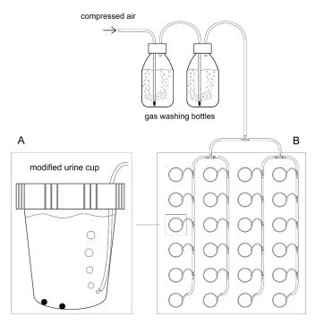
**Fig. 1.** Experimental setup of the metal leaching test. (A) Single exposure unit and (B) arrangement of the exposure units during the experiment (two shot types tested simultaneously).
