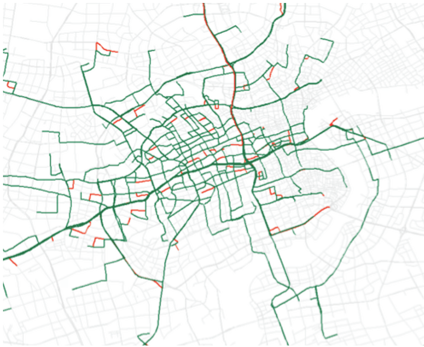
Fig.9 The matching result of trajectories of 70 taxis in Shanghai (red) on a certain day with OSM (green) using L1 Conditional Random Fields (L1-CRF) algorithm, trajectory data source: Tongji University, more details in (Yang 2016)
