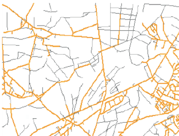
Fig.8 Integration of pedestrian roads (grey) from the Federal Agency of Cartography and Geodesy in Germany and motorways from HERE (brown): urban area (up), rural area (down) (Zhang et al. 2016)
