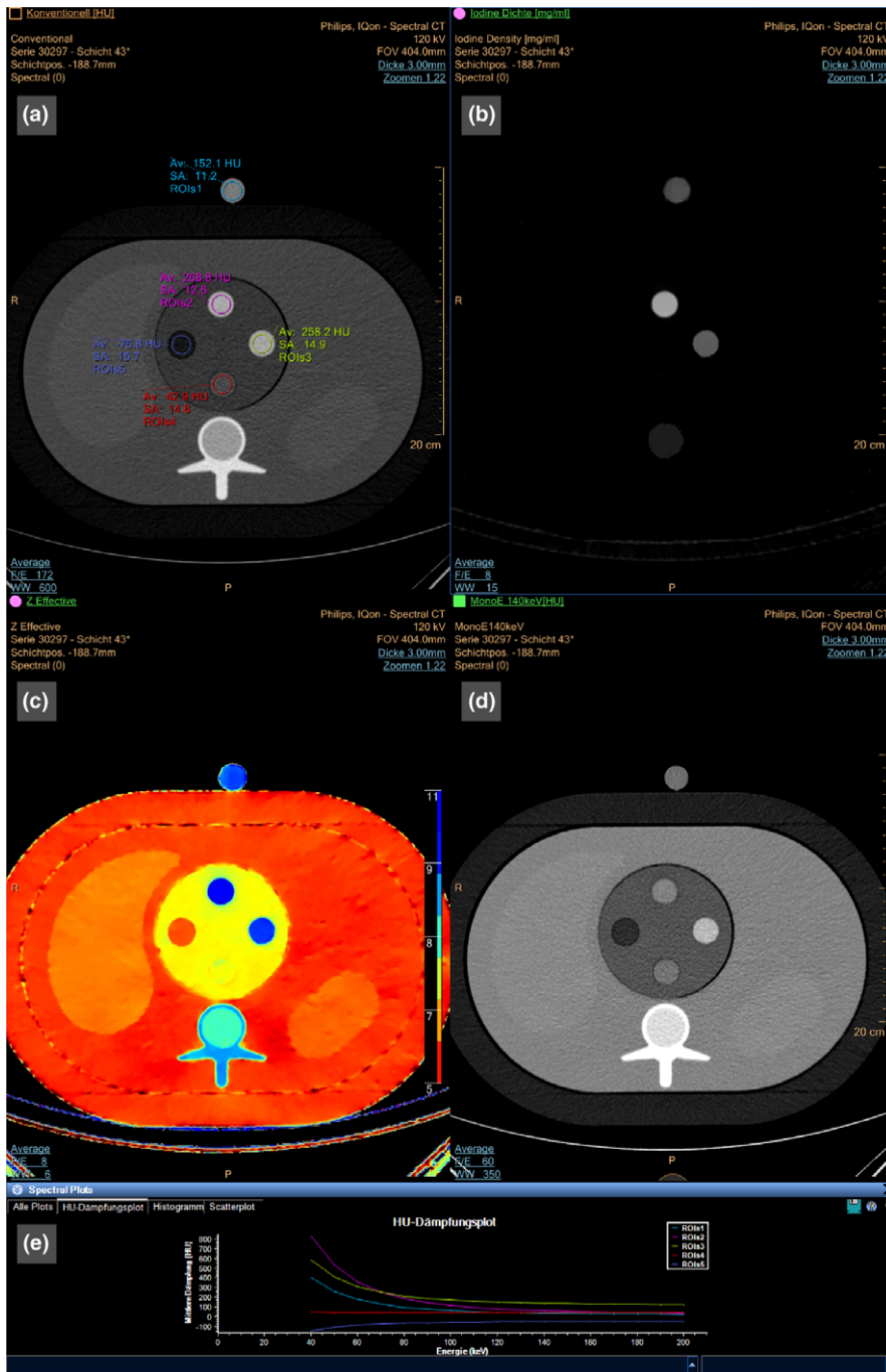
FIG. 4. Illustration of the spectral CT evaluation workflow using a commercial spectral viewer. Different selectable spectral results are shown by the toolbox. Here, the conventional image (a), an iodine density-map (b), an effective-Z map (c), and a virtual mono-energetic image (d) are shown. Additionally, energy-dependent attenuation values in the HU scale can be determined for each selected region of interest (ROI) (e).
