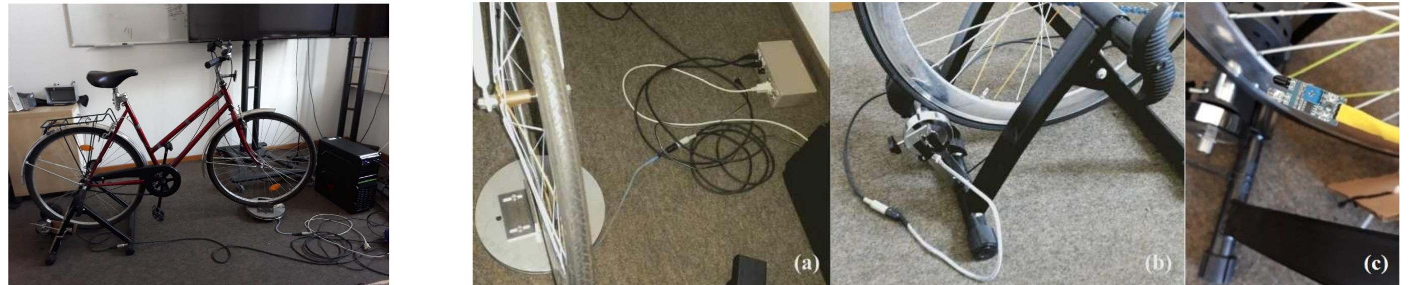
Recent and previous sensors of the bicycle simulator, with (a) rotating steering plate, (b) magnetic rotary encoder, and, (c) IR distance sensor
