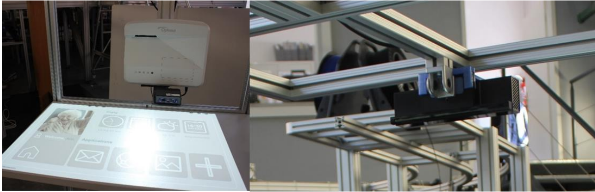
Figure 3-6 User interface and Kinect sensor in PI 2 U-MiniArc
