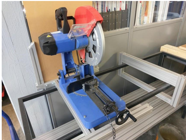
Figure 2-5 Machine to change aluminum profiles in TUM's laboratory
