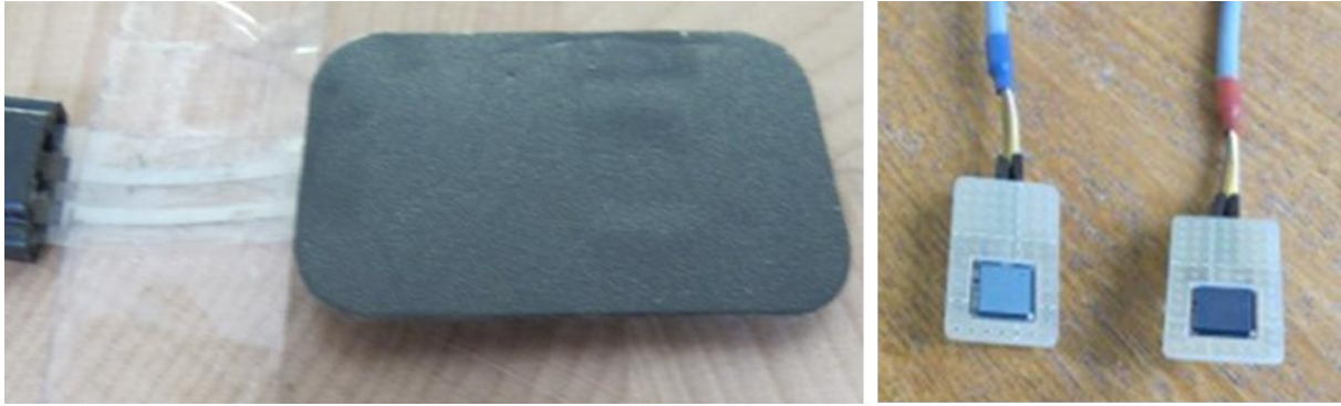
Figure 3-8 Activity monitoring sensors used in PI 2 U-Stander
