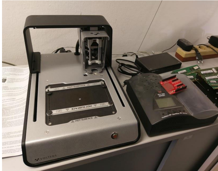
Figure 2-4 Circuit printer in TUM's laboratory
