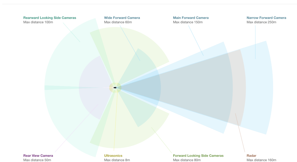
Figure 12 A visualization of the sensors and their ranges of a Tesla Model S. (Picture taken from [25])
