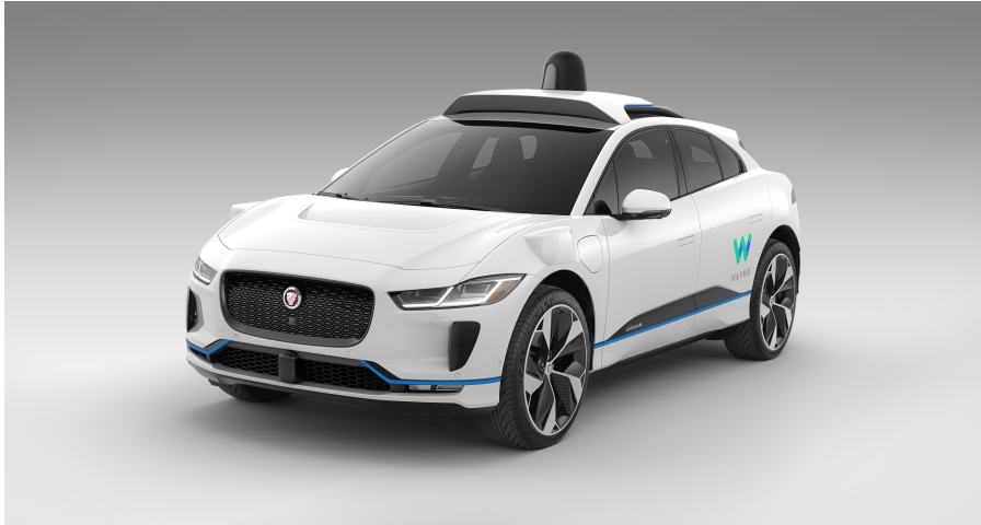
Figure 24 The electric Jaguar I-PACE with Waymos sensor suite, with fully autonomous capabilities. (Picture taken from 2 )
