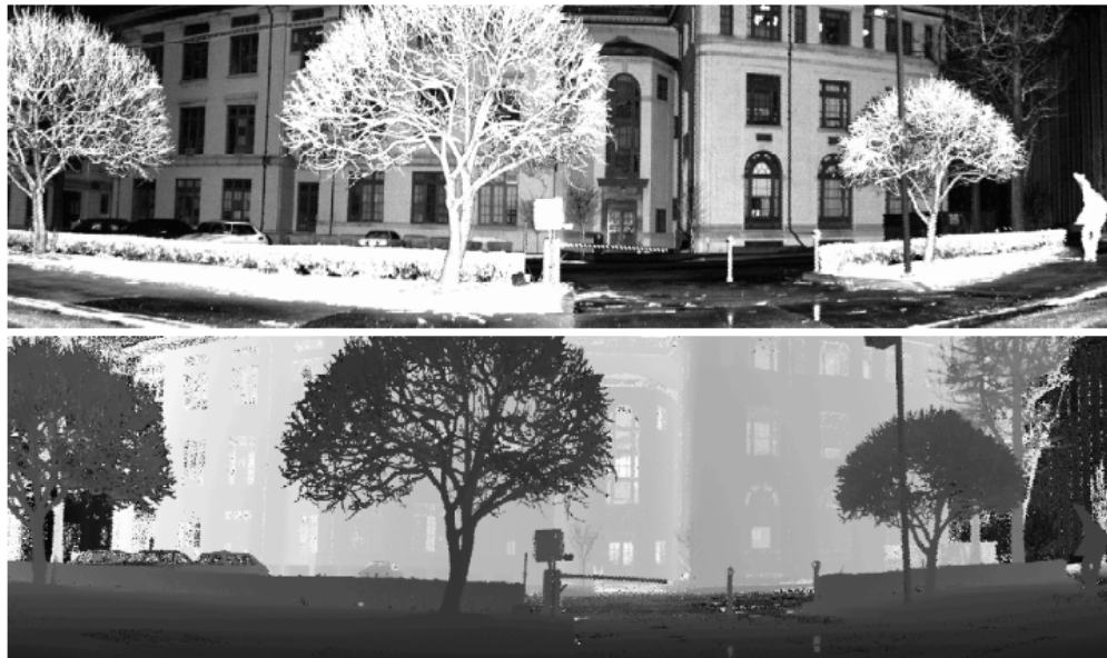
Figure 7 The data shown in the upper image represents the reflectivity data. The bottom visualization contains distance information, where darker means closer and lighter means farther. (Picture taken from [18])
