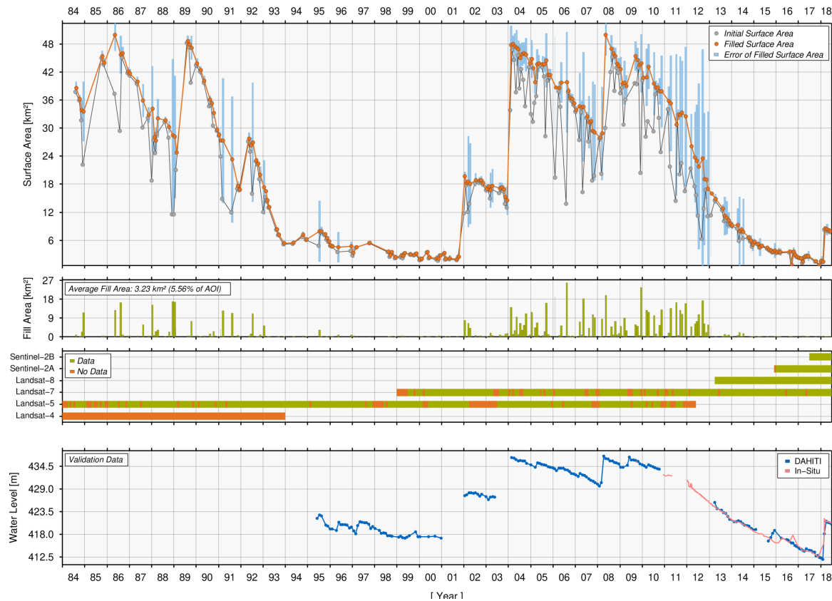
Figure 16. Water surface area time series (orange) and their errors (blue) of Poço da Cruz Reservoir. Additionally, the initial surface area with data gaps (gray) and the filled area (green) are shown. Also, the data availability of monthly optical images from Landsat and Sentinel-2 is presented. Finally, the water level time series from in situ stations and DAHITI which used for validation is shown.
