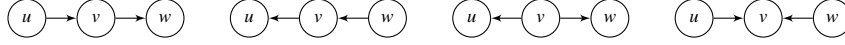
Fig. 2 The DAGs to the left of the figure are Markov equivalent; the only non-trivial element of their independence models is u \perp_{\mathcal{D}} w | v . The DAG to the right in the figure has a different independence model, since there u \perp_{\mathcal{D}} w .
