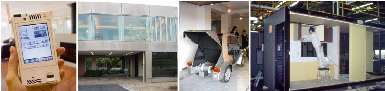
Figure 7: Toyota PAPI Dream House, a cooperative project of Toyota Home and Toyota Motor Co-operation integrating technologies from both fields. The prototype of a fully computerized building was built upon the basis of Toyota Homes steel frame units. Toyota Home is modularizing buildings and prefabricates them completely by means of the Toyota Production System in a automated factory. The prefabrication of intelligent buildings is likely to reduce costs of smart environments dramatically.
