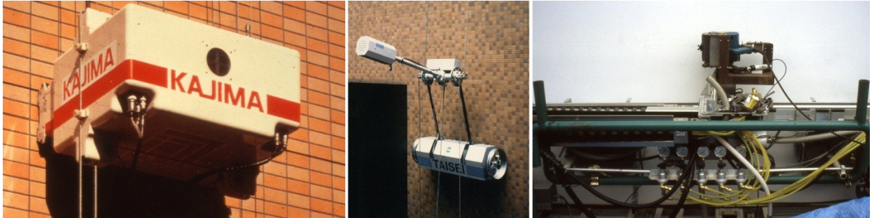
Figure 2: Left: Robot for diagnostics and automated exchange of façade elements, Kajima, Japan; Middle: Robot for façade diagnosis, Teisei, Japan, Right: Robot for multilayered painting, Tokyu
