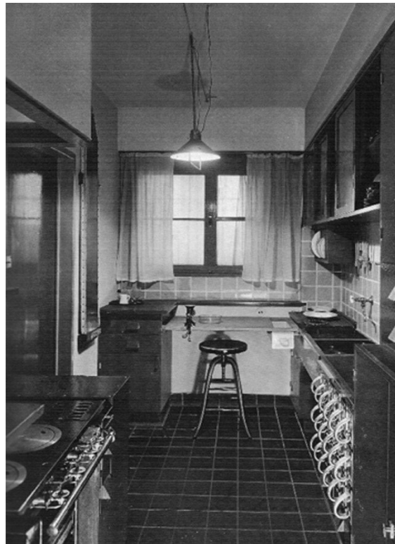
Figure 10: left: The Frankfurt kitchen transferred the principles of scientific management (Taylorism) into the German kitchen; it was developed to enable efficient flow of work on less space. Through application of Taylor’s principles the amount of movements and work steps needed to perform certain activities that are related to the higher level goals as cooking or preparing food had clearly been reduced.
