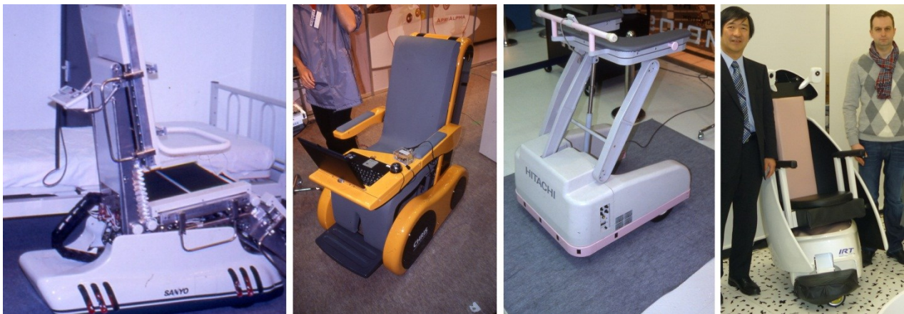
Figure 1: from left to right: mechatronic system for lifting and transfer of people; intelligent wheelchair; robotic walking frame/rollator, robotic wheelchair from IRT (Prof. Shimoyama)
