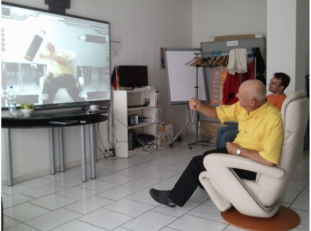
Figure 15: Sensor Chair developed within the authors’ R&D Project GEWOS. The “Fitness Chair” is measuring people’s vital signs, makes those vital signs then transparent to the user and finally try’s to activate the user to become more active (Figure 16), do sports and meet friends.
