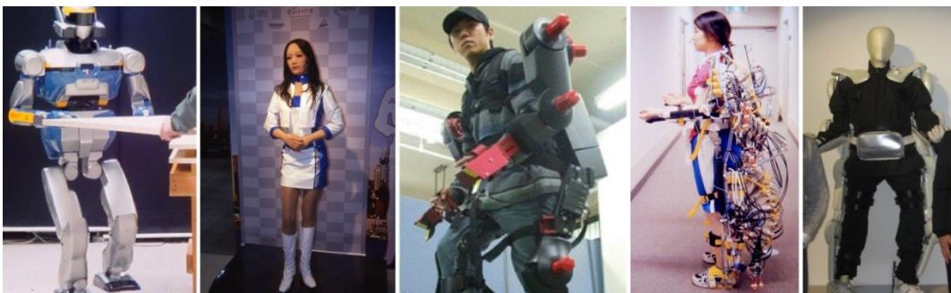
Figure 3: Left: Humanoid robots are complex autonomous systems that can adapt to changes in the environment. Right: Exoskeletons state a contrary approach, combining the flexibility and intelligence of human beings with the speed and power of robotic systems in order to allow reducing the complexity of the robotic system.
