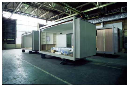
Figure 2: Sekisui Heim's legendary M1 was the first prefabricated housing model which reached an annual production of over 3000 buildings/year over several years.
