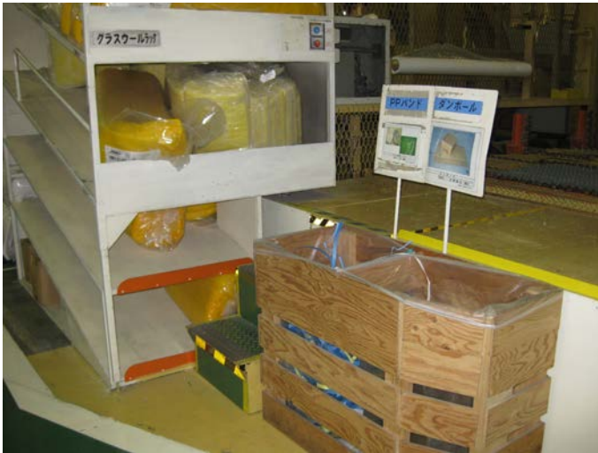
Figure 8: Materials as e.g. insulations are supplied to the factory already in the fitting sizes minimizing cutoff waste. The remaining waste is sorted fastidiously in up to 40 categories.
