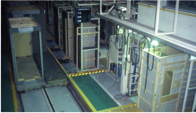
Figure 7: Insertion of prepared elements and by suppliers (e.g. Toto, Inax) prefabricated bath modules into the chassis unit.
