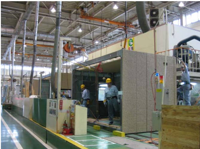
Figure 6: On the 400m production line, the steel frame units (“chassis”) pass several workstations.
