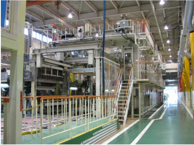
Figure 5: Automated assembly and welding of steel profiles to units.
