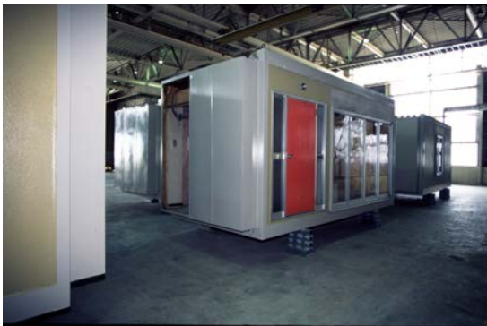
Figure 2: Sekisui Heim's legendary M1 was the first prefabricated housing model which reached an annual production of over 3000 buildings/year over several years.
