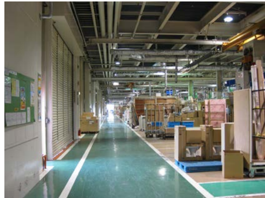
Figure 4: Exterior and Interior view of one of the two supply sides which flank the production line. The components and materials are supplied from the left side just in time and just in sequence to a small “preparation” area – from there it goes directly to the production line on the right side.
