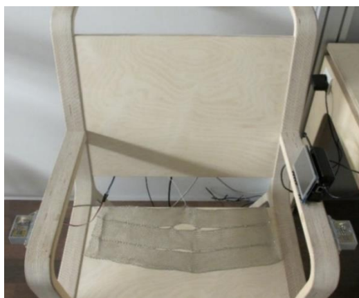
Figure 3. The capacitive Electrodes modular attached at the sides of the arm rests of a test chair.
