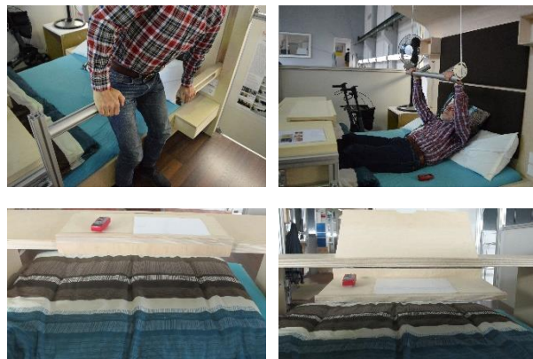
Figure 6. Left top, the unobtrusive implemented handles; Right top, the remote controlled handle; Left bottom, the integrated table on a sliding rail, which is unfolded in the figure at the right bottom.
