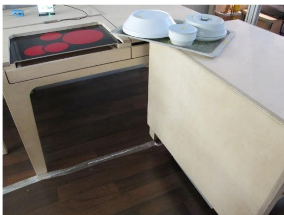
Figure 2. The mobile platform hidden in a (right) table, which can autonomous drive, controlled by a small touchscreen, which is placed on the table.
