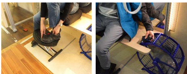
Figure 5. Left the moveable plate as support to get into the shoe; Right the ergonomically shoe shelf
