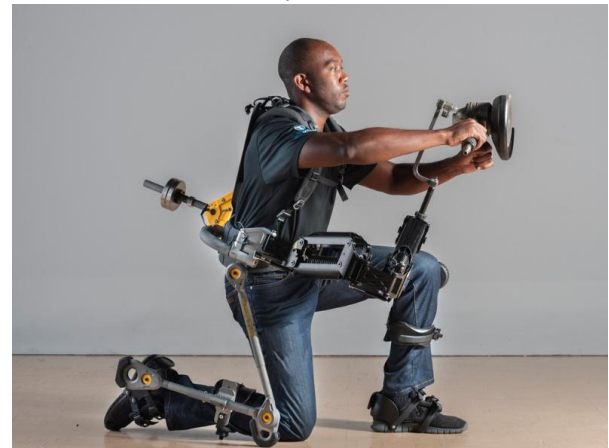
Fig.4. FORTIS exoskeleton, created by Lockheed Martin, can boost worker productivity up to 27 times. (Image: Photo Courtesy of Lockheed Martin. Copyright 2015)
