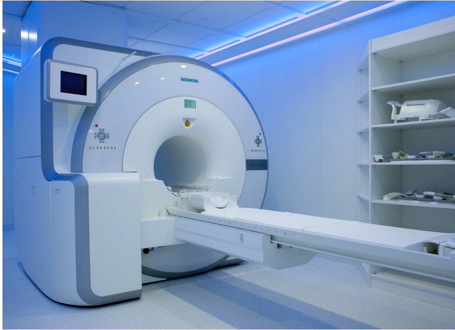
Figure 1.3: The Siemens Biograph mMR fully-integrated PET/MR scanner. Image courtesy of www.siemens.com/press .
