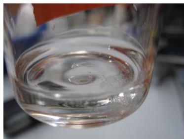
a) Distilled bimenthyl fraction (neat); early stage of crystallization, ca. 2 x original size.
